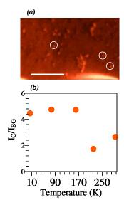
Fig. 4. (a). SEM of typical QD coverage for the results in Fig. 3, showing single QDs at concentrations of <1000 per  $\mu$ m<sup>2</sup>. Scale bar: 100 nm (b) QD intensity contrast (I<sub>c</sub>) over the background (I<sub>BG</sub>) as a function of temperature.
