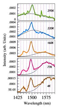
Fig. 3. PL spectra of dots at cavity (r = 124 nm) at 4, 77, 160, 220 and 295 K, showing the cavity mode being decorated at all temperatures. Gaussian fits to the QD PL spectrum, as well as Lorentzian fits to the cavity line are also shown.
