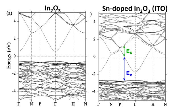
Large carrier concentration desired for better conductivity, increases optical absorption
