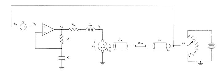
The angular position of the motor shaft is detected by a variable resistor which provides a voltage  $v_o$  proportional to the angle, such that  $v_o = -K_o\theta_o$ . Draw the most detailed block diagram of the system, where  $v_i$  is the input, and  $\theta_o$  is the output. Show all the variables  $v_i$ ,  $v_o$ ,  $v_j$ ,  $v_a$ ,  $v_b$ ,  $i_a$ ,  $\tau$ ,  $\theta_m$ , and  $\theta_o$  on the block diagram. (25pts)
