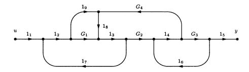
In drawing the signal flow graph, the unity gains are subscribed for easy tracking of the gain expressions. The forward path gains are
