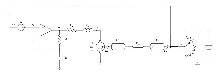
The angular position of the motor shaft is detected by a variable resistor which provides a voltage  $v_o$  proportional to the angle, such that  $v_o = -K_o\theta_o$ . Draw the most detailed block diagram of the system, where  $v_i$  is the input, and  $\theta_o$  is the output. Show all the variables  $v_i$ ,  $v_o$ ,  $v_j$ ,  $v_a$ ,  $v_b$ ,  $i_a$ ,  $\tau$ ,  $\theta_m$ , and  $\theta_o$  on the block diagram.
