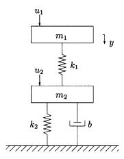
(a) Obtain the transfer matrix of the system assuming that the external forces  $u_1$  and  $u_2$  are the inputs, and the displacement y is the output.
