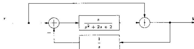
Obtain a state-space representation of the system without any block-diagram reduction. (20pts)
