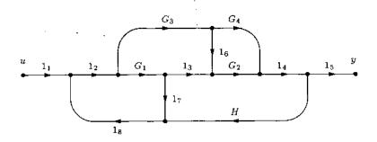
In drawing the signal flow graph, the unity gains are subscribed for easy tracking of the gain expressions. The forward path gains are
