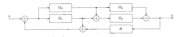
Solution: If we choose to use the block diagram reduction, best approach is to reduce the block diagram step by step, until we obtain the transfer function.
