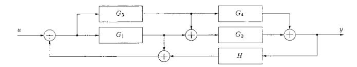
3. Consider the following block diagram representation of a control system, determine the transfer matrix of the system. (25pts)
