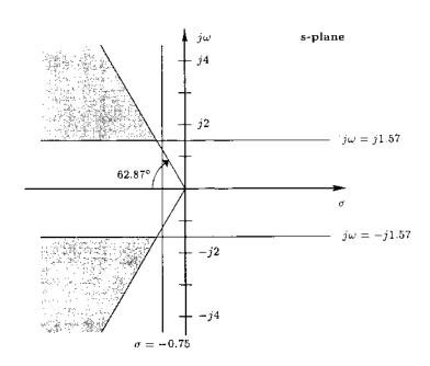
The restriction  $\sigma \leq -0.75$  could be unnecessary, if the straight line that is making 62.87° with the negative real axis intersects the  $j\omega = j1.57$  line to the left of the  $\sigma = -0.75$  line. That intersection is at  $-1.57/\tan(62.87^\circ) = -0.80$ . So, the specification that resulted in the restriction  $\sigma \leq -0.75$  is unnecessary. In other words, the specification  $t_{5\%s} \leq 4 \,\mathrm{s}$  is unnecessary.
