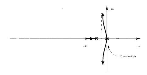
As we observe from the root-locus diagram, any positive value of K will generate asymptotically stable closed-loop poles. Therefore, the simplest controller is
