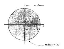
The equi-distance points from the origin designate constant value for  $\omega_n$ . As a result, the shown shaded area is represented by
