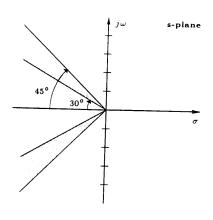
A straight line originating from the origin designates a constant  $\zeta$  value, where  $\cos^{-1}(\zeta)$  is the acute angle between the line and the negative real axis. So for the shaded area shown, we have
