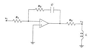
Assume that  $R_1 = 1\Omega$ ,  $R_2 = 2\Omega$ ,  $R_3 = 4\Omega$ , C = 1F, and L = 2H. Only the capacitor and the inductor are sensitive to temperature changes; such that the sensitivity of the capacitance with respect to temperature  $\mathcal{S}_T^C = 5$ , and the sensitivity of the inductance with respect to temperature  $\mathcal{S}_T^L = 4$ . Determine the sensitivity of the transfer function  $V_o(s)/V_i(s)$  with respect to the temperature. (20pts)
