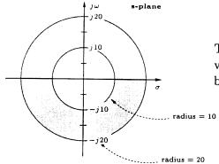
The equi-distance points from the origin designate constant value for  $\omega_n$ . As a result, the shown shaded area is represented by
