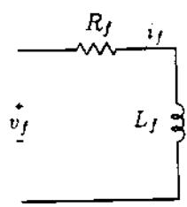
$$\begin{aligned} L_f \frac{di_f}{dt} + R_f i_f &= v_f \\ (L_f s + R_f) I_f(s) &= V_f(s) \\ I_f(s) &= \frac{1}{L_f s + R_f} V_f(s) \end{aligned}$$
