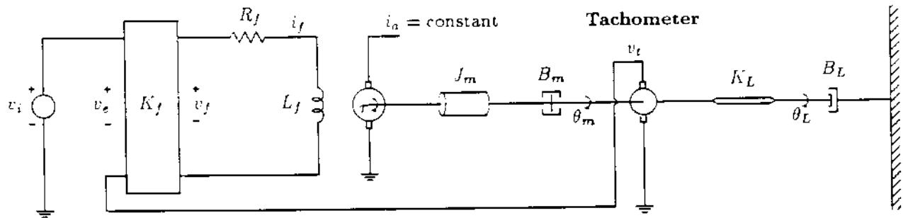
Here, the ideal amplifier at the field winding of the motor has a gain of  $K_f$ . Assuming that the output voltage of the tachometer is proportional to the angular speed, such that  $v_t = K_t \omega_m$ , draw the most detailed block diagram of the system. Also assume  $v_i$  is the input,  $\theta_L$  is the output, and show all the variables  $v_i$ ,  $v_e$ ,  $v_f$ ,  $i_f$ ,  $\tau$ ,  $\omega_m$ ,  $\theta_m$  and  $\theta_L$ . (30pts)
