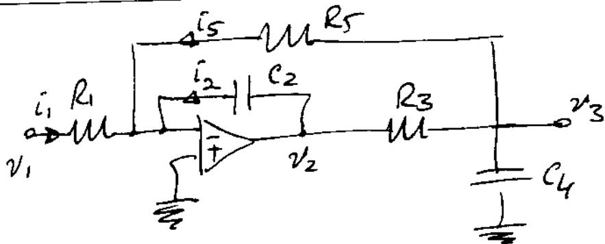
$$a_{11} \quad i_1 = \frac{1}{R_1} v_1$$
