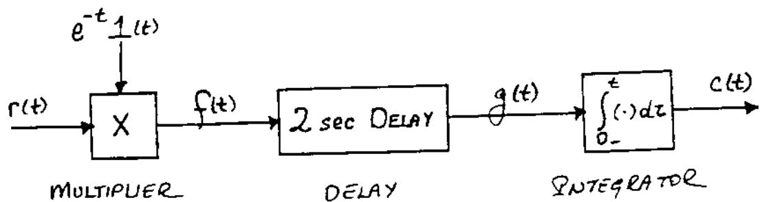
determine the input signal  $r(t)$ , where  $\mathcal{L}[c(t)] = \frac{3e^{-2s}}{s[(s+1)^2 + 9]}$ . (15 pts)
