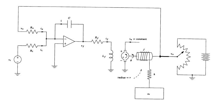
The angular position of the motor shaft is detected by a variable resistor which provides a voltage  $v_o$  proportional to the angle, such that  $v_o = K_o \theta$ . Draw the most detailed block diagram of the system, where  $v_i$  is the input, and  $\theta$  is the output. Show all the variables  $v_i$ ,  $i_i$ ,  $v_o$ ,  $i_o$ , i,  $v_f$ ,  $i_f$ ,  $\tau$ , and  $\theta$  as well as the displacement(s) associated with the mass-spring components on the block diagram.
