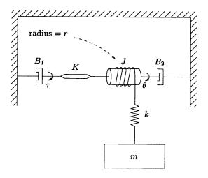
(a) Obtain the transfer function of the system assuming that the external variable  $\tau$  is the input, and the angle  $\theta$  is the output. Assume that the spring with the spring constant k is stretched due to the gravity prior to the application of the torque  $\tau$ .
