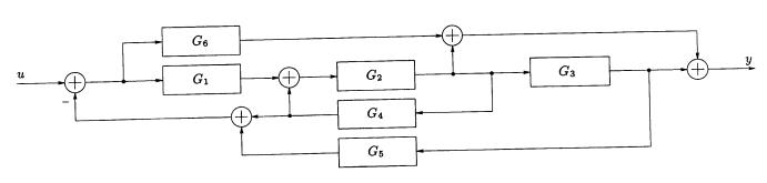
**Solution:** If we choose to use the block-diagram reduction, best approach is to reduce the block diagram step by step, until we obtain the transfer function.
