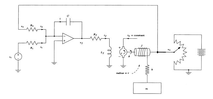
The angular position of the motor shaft is detected by a variable resistor which provides a voltage  $v_o$  proportional to the angle, such that  $v_o = K_o \theta$ . Draw the most detailed block diagram of the system, where  $v_i$  is the input, and  $\theta$  is the output. Show all the variables  $v_i$ ,  $i_i$ ,  $v_o$ ,  $i_o$ , i,  $v_f$ ,  $i_f$ ,  $\tau$ , and  $\theta$  as well as the displacement(s) associated with the mass-spring components on the block diagram. (25pts)
