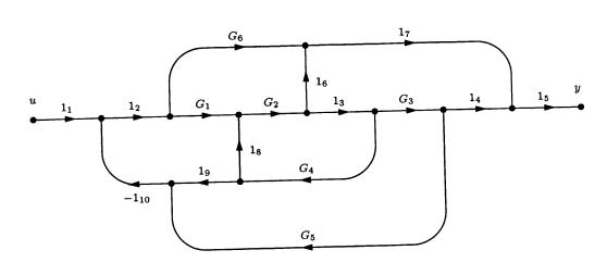
In drawing the signal flow graph, the unity gains are subscribed for easy tracking of the gain expressions. The forward path gains are
