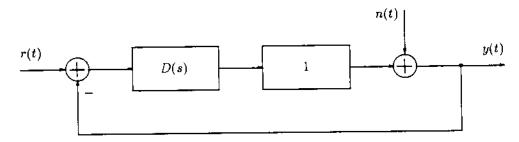
Design the simplest controller D(s), so that the output, y(t), follows a sinusoidal input, r(t), with a frequency of 1 rad/sec, and it rejects a sinusoidal noise, n(t), with a frequency of 4 rad/sec. (30pts)
