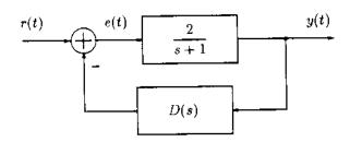
4. A modified PD controller is to be designed for the following system. Determine the range of controller constants  $K_P$  and  $K_D$  for an asymptotically stable system. (25pts)
