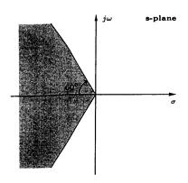
A straight line originating from the origin designates a constant  $\zeta$  value, where  $\cos^{-1}(\zeta)$  is the acute angle between the line and the negative real axis. So for the shaded area shown, we have
