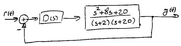
(a) Design a D(s), where the order of the closed-loop system is at most three.
