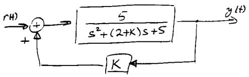
(a) Construct the root-locus diagram as K goes from 0 to  $\infty$ .
