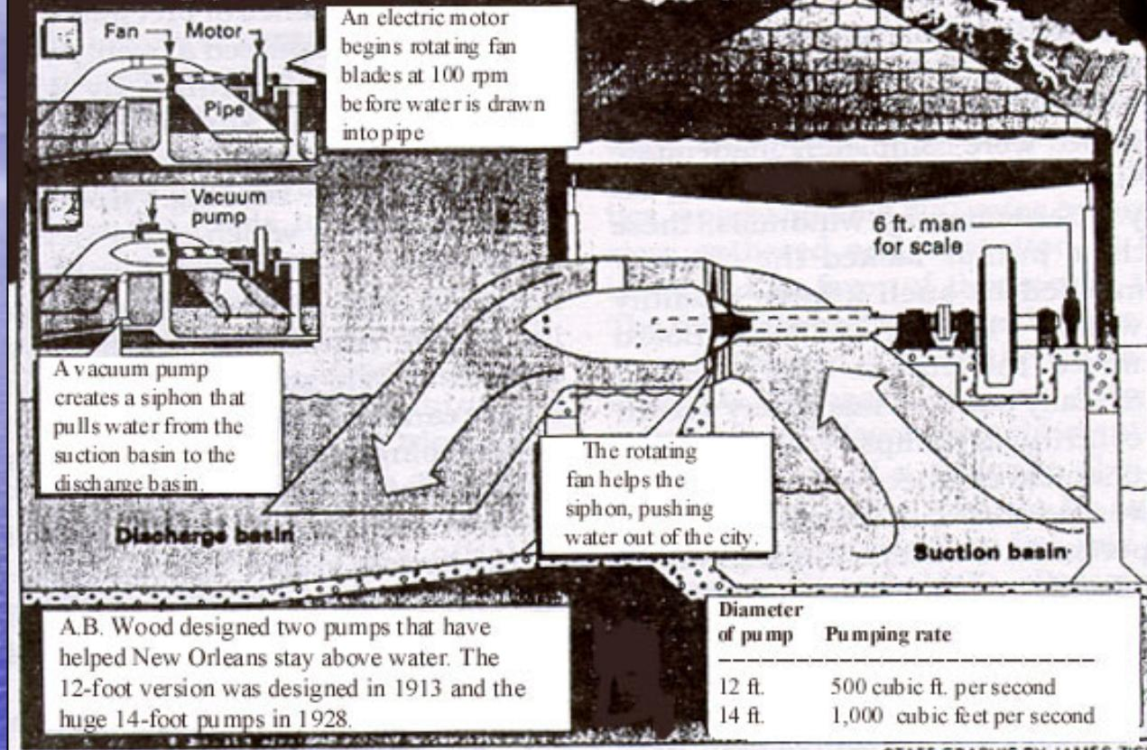
This 1920s drawing shows the arrangement of a Wood screw pump, which uses a powerful siphon action to lift water into the drainage canals, where it flows by gravity to Lake Ponchartrain. The City's 21 pump stations can lift 47,000 csf of water. Prior to Katrina, it had only been overwhelmed on a few occasions, in 1978 and again, in 1995.
