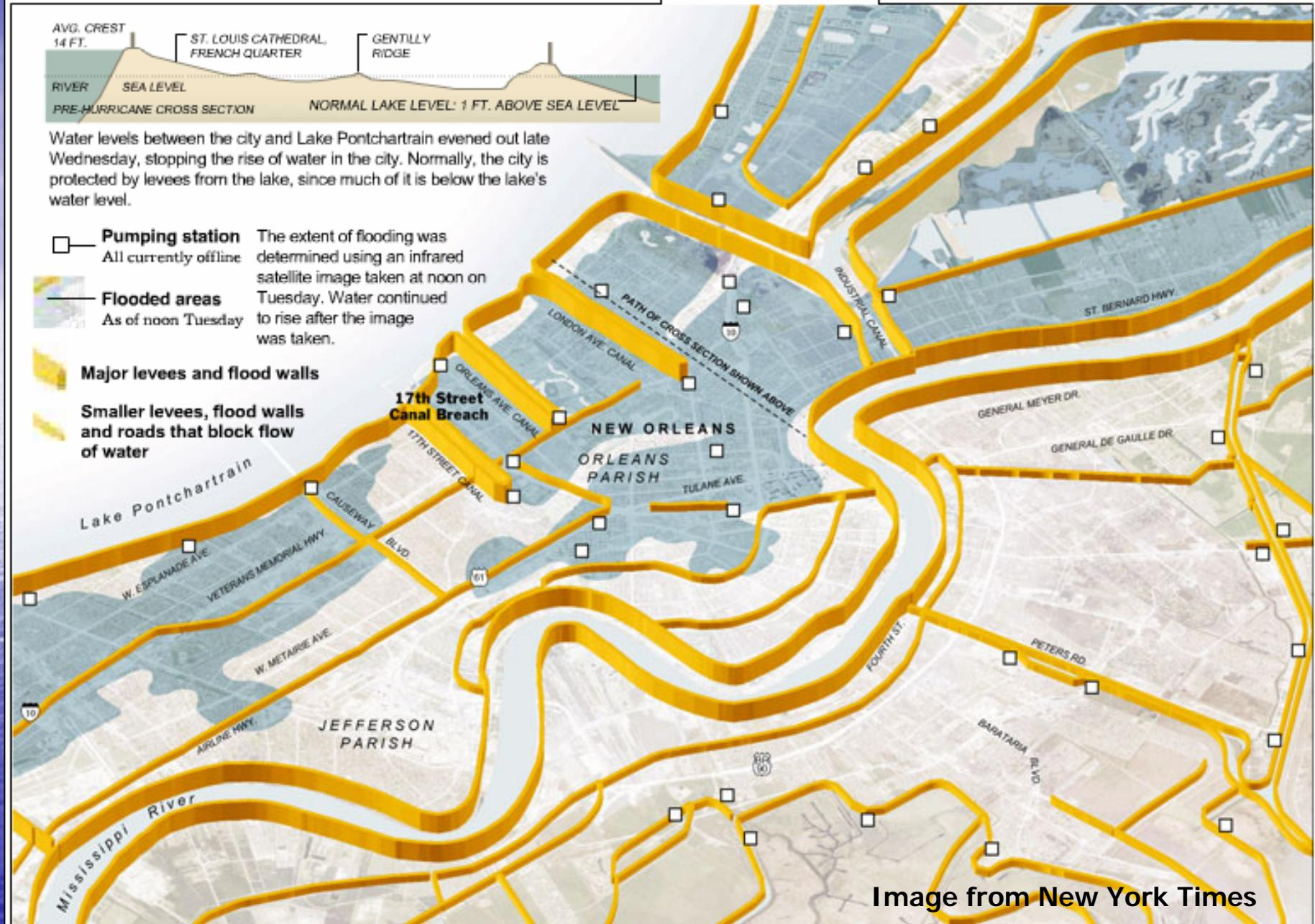
**A complex network of levees protected the city from flooding, but it quickly failed on August 29, 2005, when water levels rose.**
