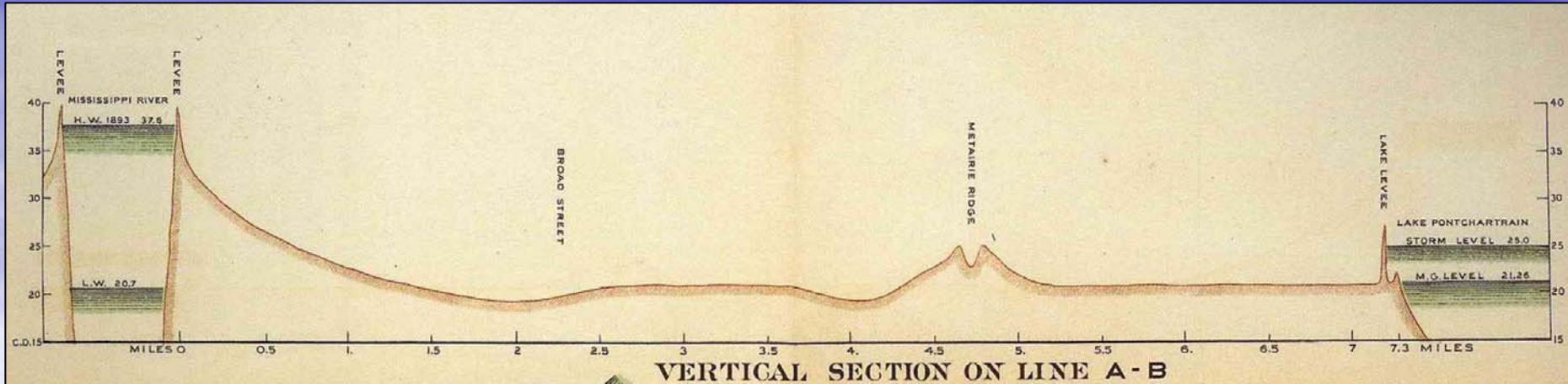
Cross section through New Orleans in 1895. The Mississippi River's natural levees form the highest ground in New Orleans. **Metarie and Gentilly Ridges** are recent distributary channels, lying about 3 to 6 feet above the adjacent ground. The earliest levees along Lake Ponchartrain (far right) were erected in the 1890s; then enlarged considerably in 1931-32, when the concrete seawall was built  $\frac{1}{2}$  mile into Lake Ponchartrain and backfilled with the Lakshore Landfill.
