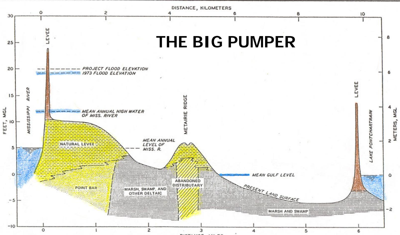
Much of New Orleans lies below sea level, Lake Ponchartrain, and the Mississippi River, making it particularly vulnerable to flooding. Mississippi levee 24.5 feet; Pontchartrain levee 13.5 feet.
