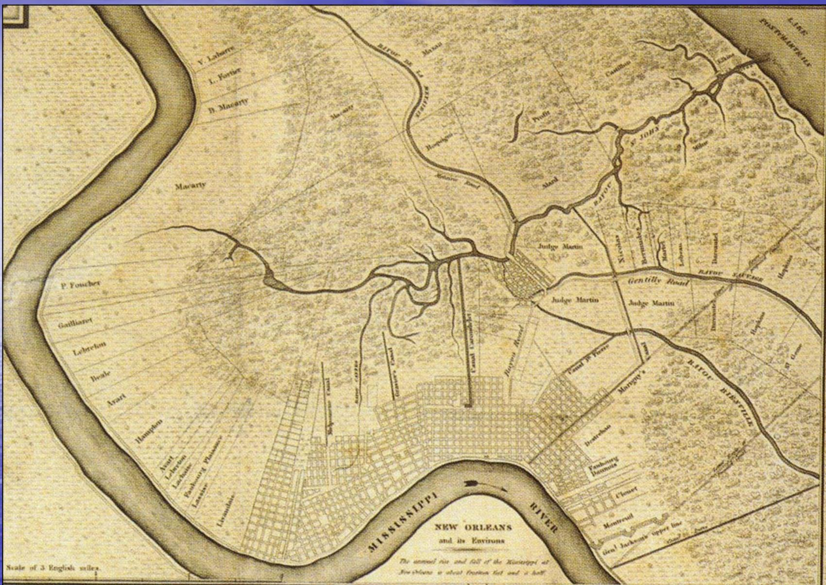
The **Old Basin drainage canal** was excavated in the **1790s**. This shows the systems of drainage ditches and canals established by 1829, leading to Bayou St. John.
