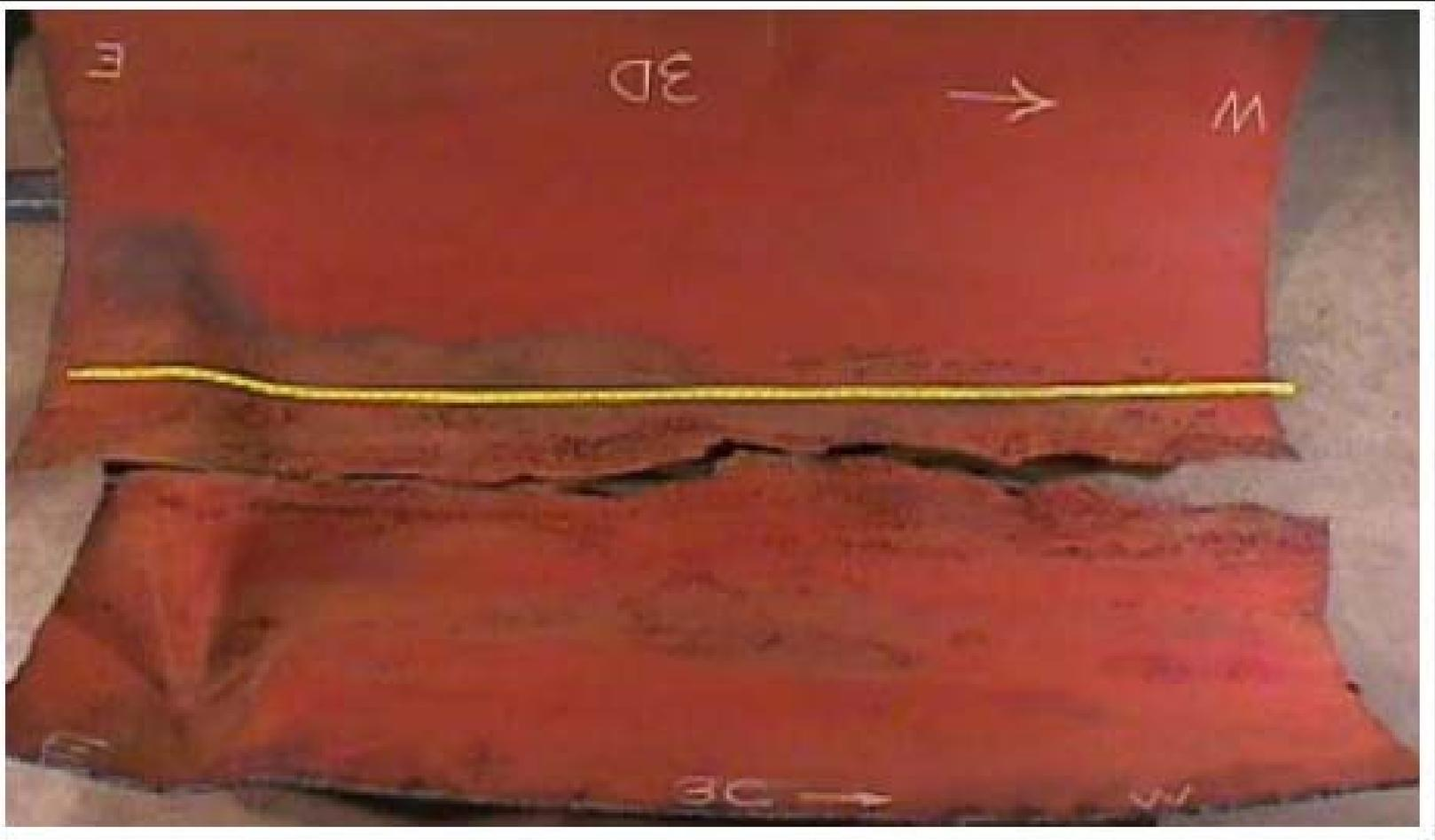
Fractured section of Pipeline 1103. Examination of the four sections of pipe ejected from the blast crater revealed extensive corrosion along the inside of the bottom of the pipe, reducing cross sectional thickness by 72%. Affected length was about 22 ft. This pitting was caused by **acid-producing bacteria**.
