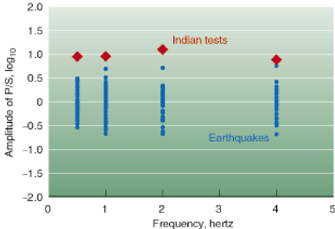
Figure 3. P-to-S amplitude ratios versus frequency for the Indian nuclear test (diamonds) and nearby earthquakes (circles). Note that the P- to S-wave ratios are higher for the Indian test than for the earthquakes.
