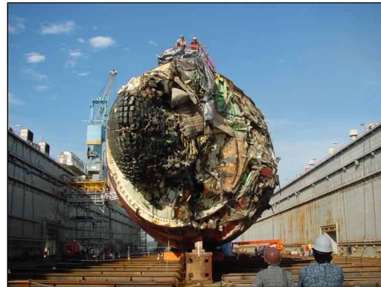
**Nuclear powered submarines are designed to withstand considerable battle damage. These views show massive damage to forward section of *USS San Francisco* (SSN 711) on Feb 12, 2005 when she collided with seamount off Guam. Only 1 crewman killed and 98 injured, 23 seriously, out of 137 aboard.**
