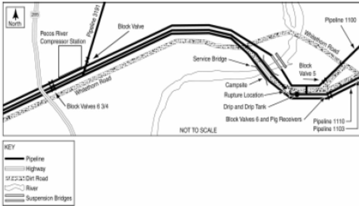
**The explosion occurred adjacent to five bridges that convey four natural gas pipelines across the Pecos River about 4.5 miles north of the New Mexico-Texas border. The fifth bridge is for a service road along the buried pipelines. Note nearby compressor station.**
