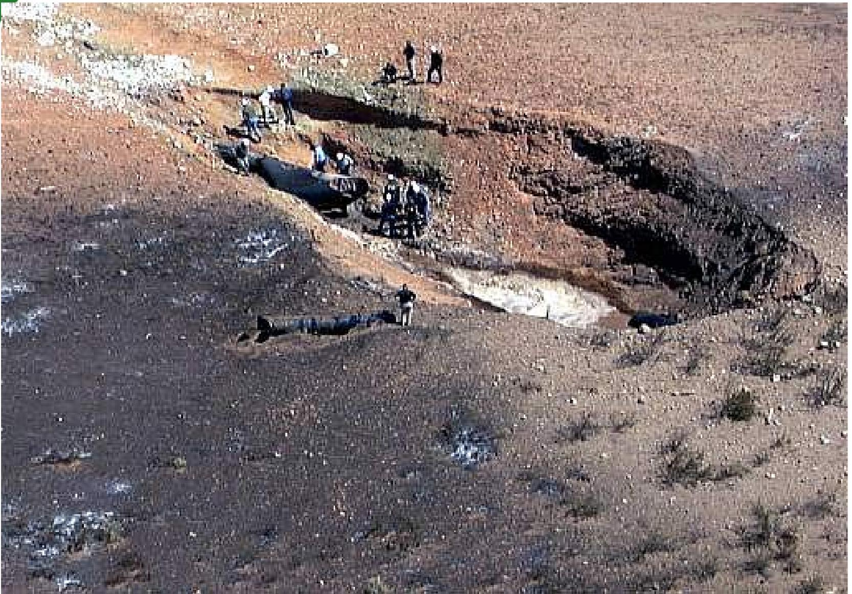
**The explosion created a 51 ft wide crater along 113 lineal feet of Pipeline 1103. 49 lineal feet of pipeline was ejected from the crater in four segments.**
