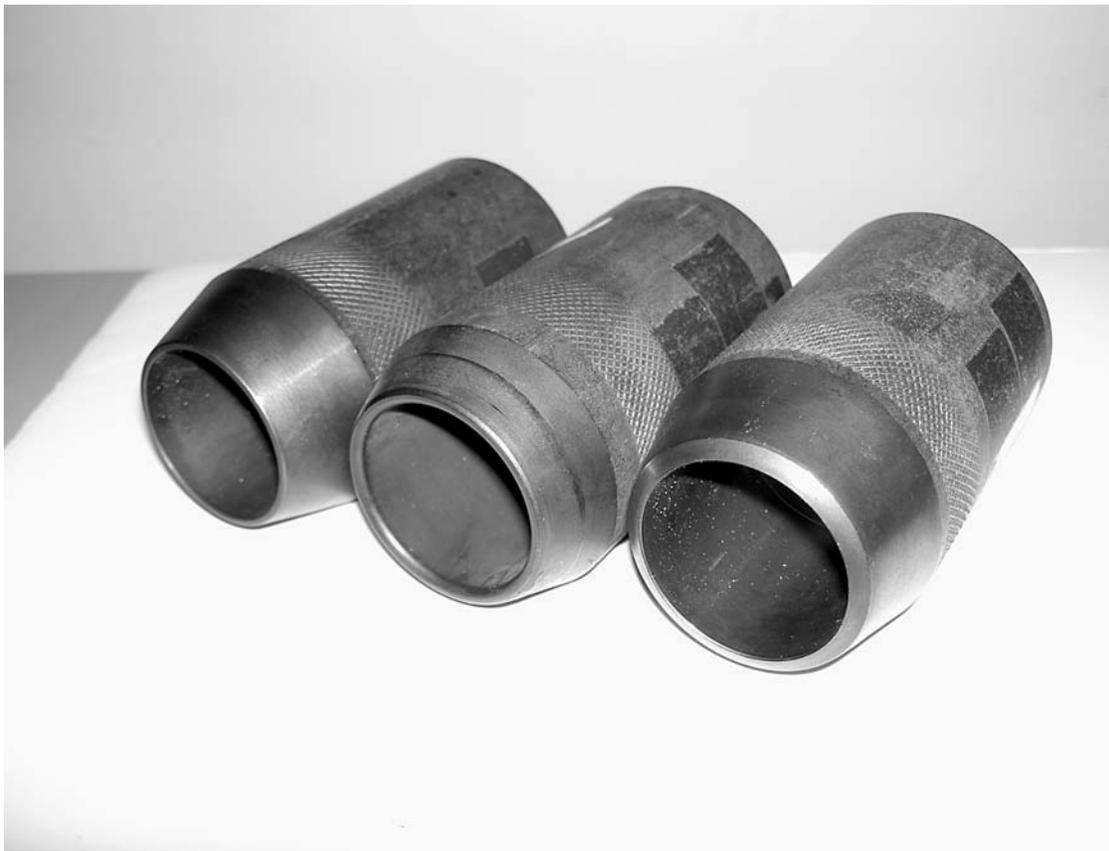
Figure 3. Drive samplers usually employ three types of cutting heads, or shoes, shown here. The sharp tapered heads are intended for soil sampling, while the more blunt tips are designed for greater longevity when sampling granular soils.
