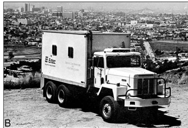
Figure 12. (A, left). Cone tip exposed beneath truck, just before being advanced into the ground at a rate between 1 and 2 cm/s. The cone has an area of either 10 or 15 cm<sup>2</sup> and is typically advanced in 1-m increments because the rods are of that length. (B, right) A Hogentogler Cone Penetrometer Test (CPT) rig operated by Ertec in Long Beach, CA. Truck-mounted rigs weigh about 18 tons and are capable of exerting considerable normal force on the advancing rods.
