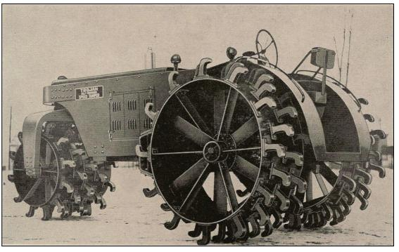
Right - Ragland's power driven Trojan Self Propelled Speed Tamper roller, produced by Contractor's Machinery Co. of Batavia, NY in the 1930s. It weighed 8,740 lbs and the club headed teeth exerted a 250 psi contact pressure.
