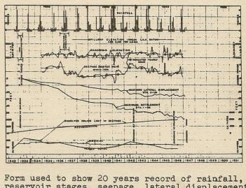
Form used to show 20 years record of rainfall, reservoir stages, seepage, lateral displacement and settlement of crest of dam, and dissolved solids in seepage water, together with earthquake, repair, grouting and related data.
