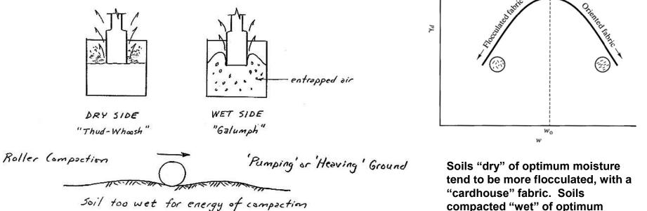
Soil simply deforms in lieu of consolidating Would have to squeeze water out of pores before further compaction could be accomplished compacted "wet" of optimum moisture tend to be more compact, with lower void ratio
