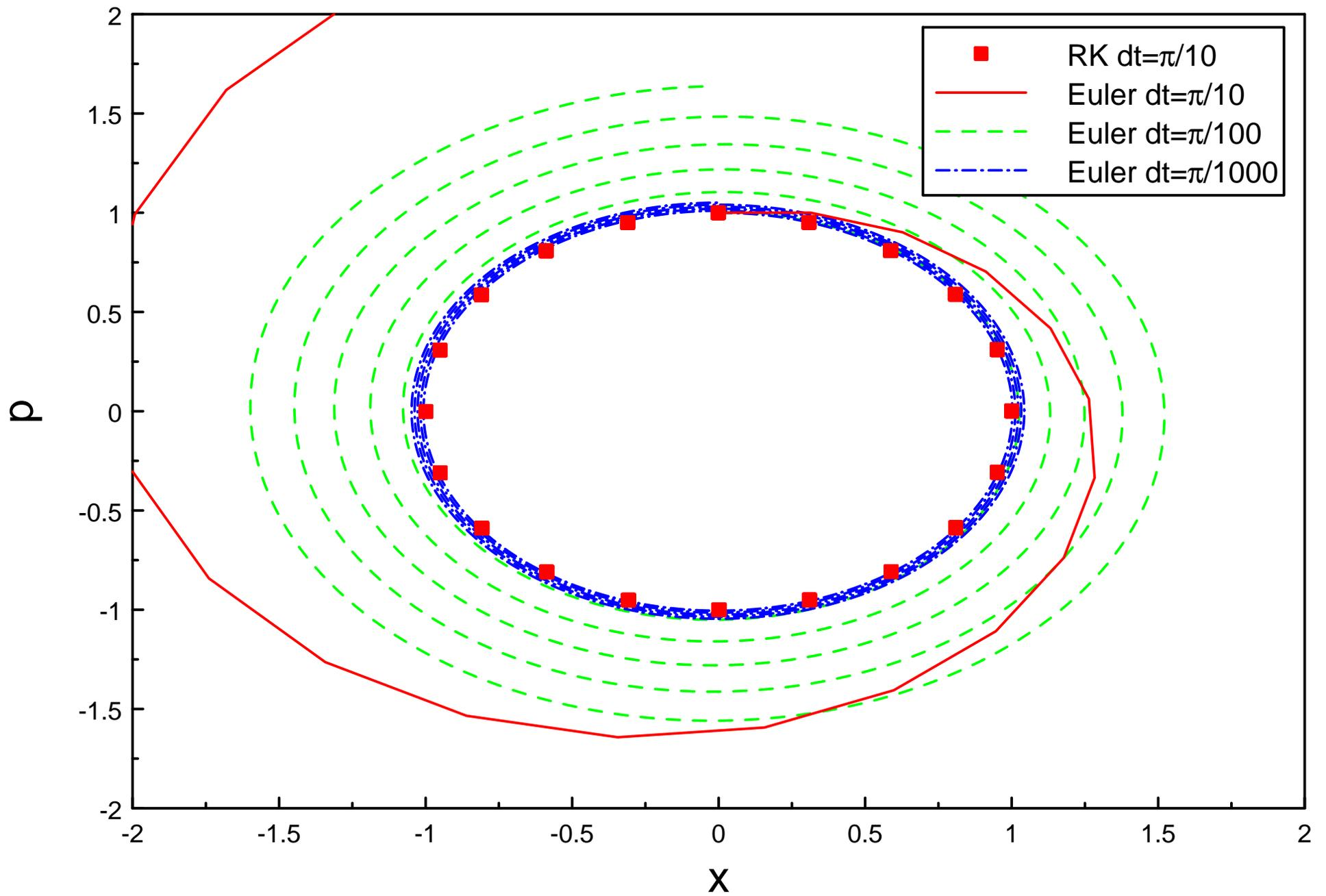
Phase space plot for comparison of Euler and Runge-Kutta methods for integrating the equation of motion of an harmonic oscillator  $d^2x/dt^2 + x=0$
