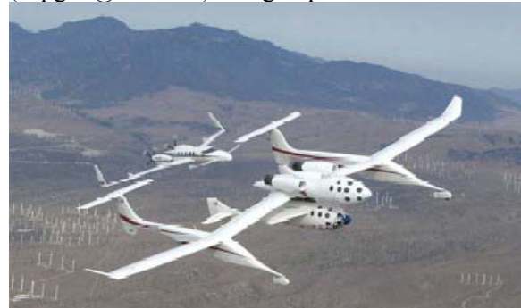
Scaled Composites White Knight launch aircraft carrying SpaceShipOne followed by a Beech Starship chase aircraft
