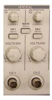
The Menu button activates the selection menu on the right side of the display, and switches its selections to those appropriate for the input channel. For this scope you have the following settings that can be accessed.
