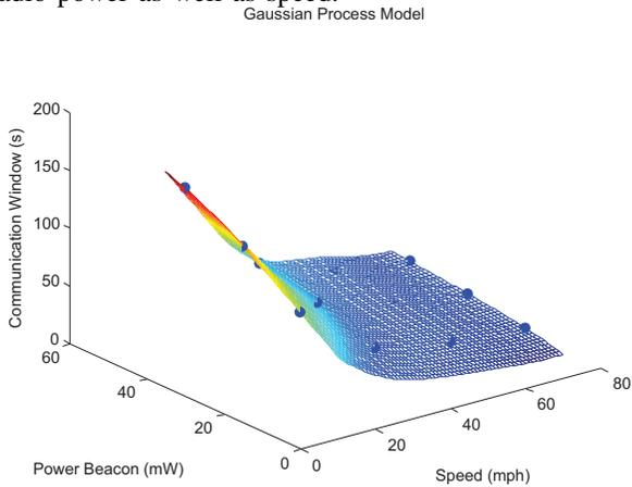
Figure 2. Surrogate Model using Gaussian Process
