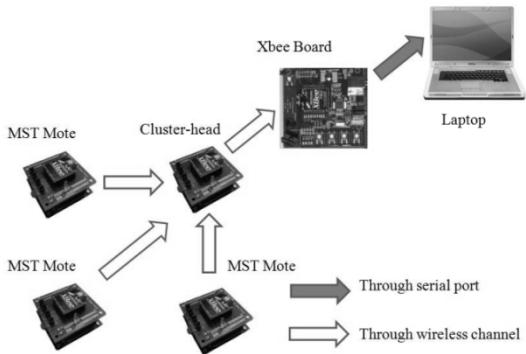
Figure 5. Hardware architecture
