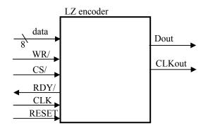
Fig. 1. Block diagram of the LZ encoder.
