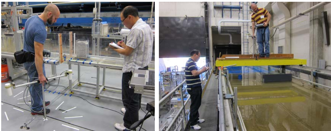
(a) Small flume tests (b) Small-scale bridge pier tests in large flume Fig. 6 Measurement with a magnetometer
