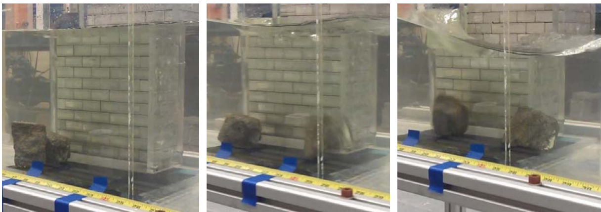
(a) Rocks at rest (b) 1 st rock rotating (c) 2 nd rock moving Fig. 5 Movement of two rocks at various flow velocities
