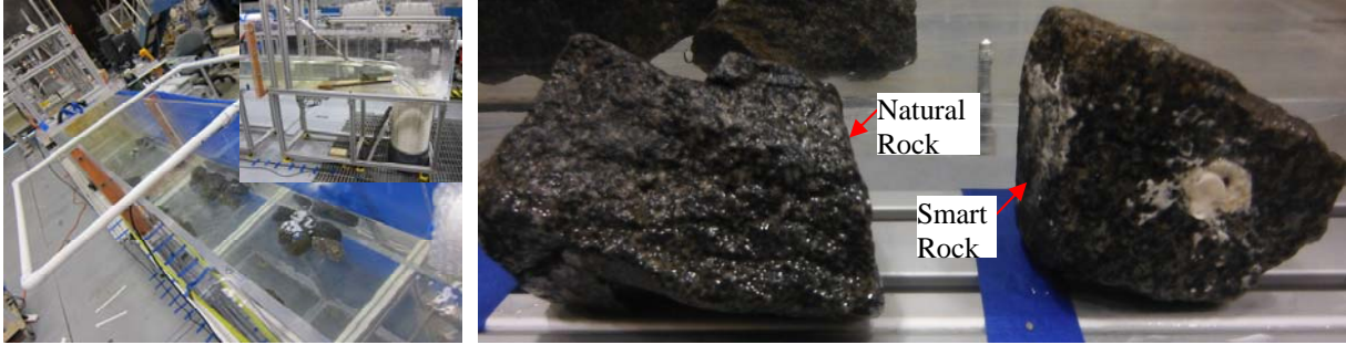
(a) Small flume at TFHRC (b) Natural rocks with and without an embedded magnet Fig. 4 Overview of the small flume and a passive smart rock
