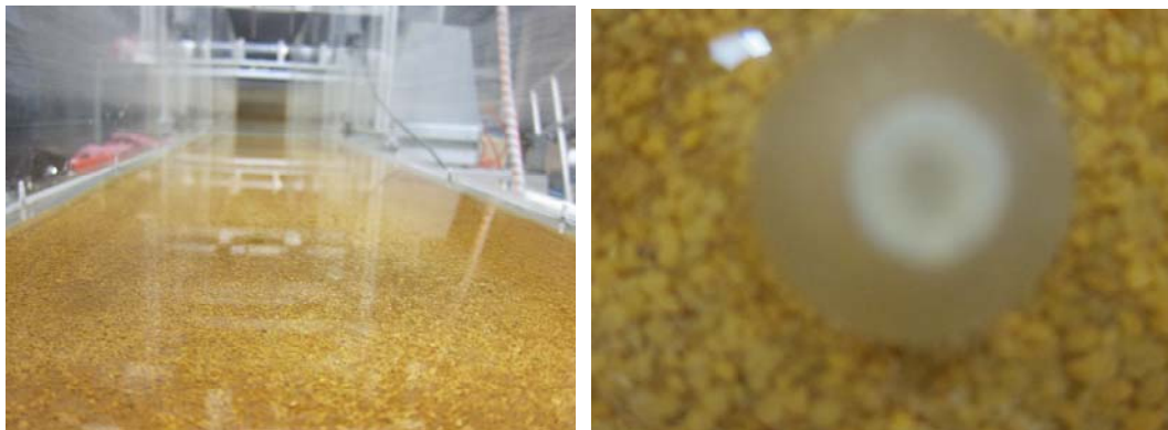
(a) Bottom texture of the flume (upstream) (b) Acrylic ball with an embedded magnet Fig. 1 Minimum velocity test of various passive smart rocks
