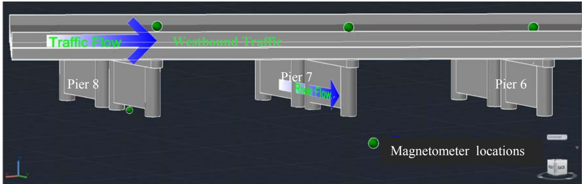
Figure 3.45 I-44 Roubidoux Creek Bridge, Pulaski County, MO Test Layout
