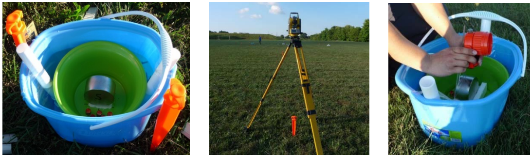
(c) Primitive APSS (d) Total Station for Positioning (e) Prism for Precision Positioning
