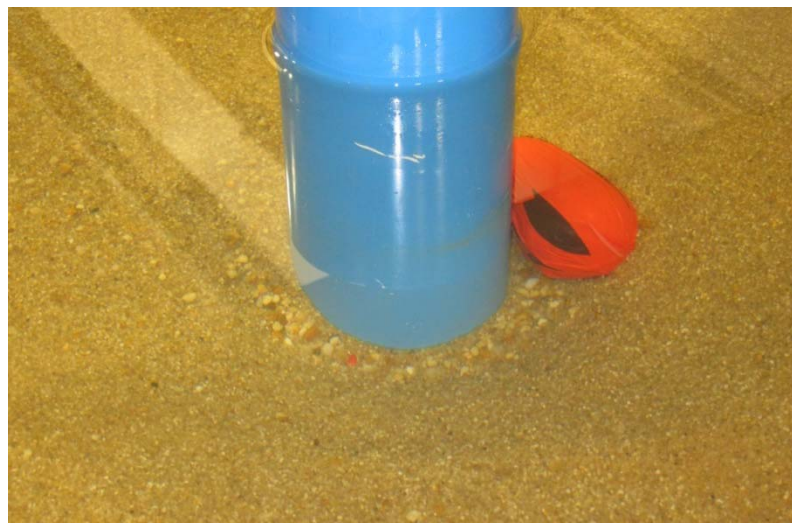
Figure 4.31 An Active Smart Rock Deployed around the Circular Pier in Large Flume
