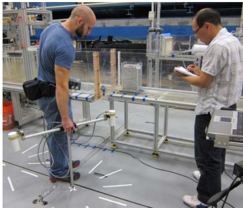
Figure 3.25 Measurement with a Magnetometer in the Small Flume
