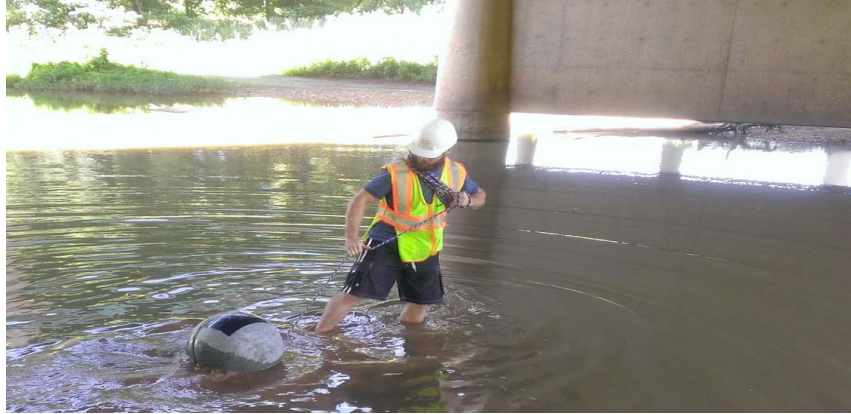
Figure 4.43 Deployment of an Active Smart Rock near the I-44 Bridge Pier
