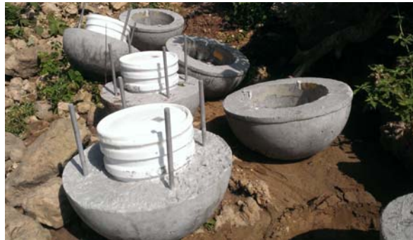
Figure 4.45 Field Assembling of Active Smart Rocks at the US63 Bridge Site
