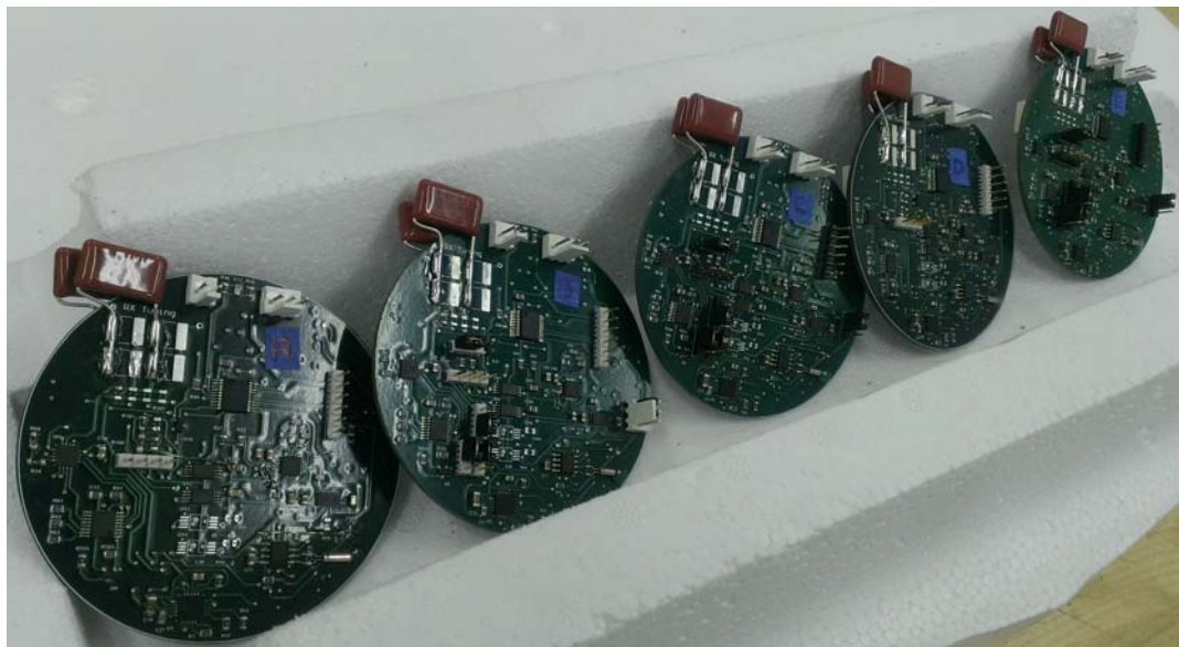
Figure 4.44 Five Core Electronic Boards Ready for Inclusion in Smart Rocks
