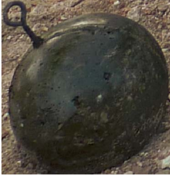
Figure 3.50 Retrieved Passive Smart Rock after the August 7, 2013 Flood
