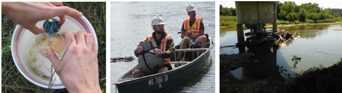
Fig. 8 Smart rock v2.4 board and deployment near the scour-susceptible pier
