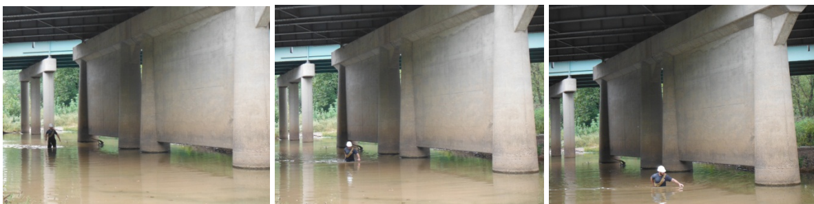
Fig. 4 Movement simulation by manually dragging a prototype smart rock near a bridge pier
