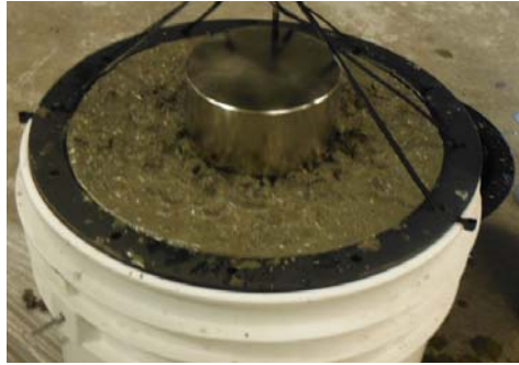
(a) Bottom half a concrete encasement (b) Top half of a concrete encasement Fig. 2 Placement of a magnet and casting of spherical concrete block
