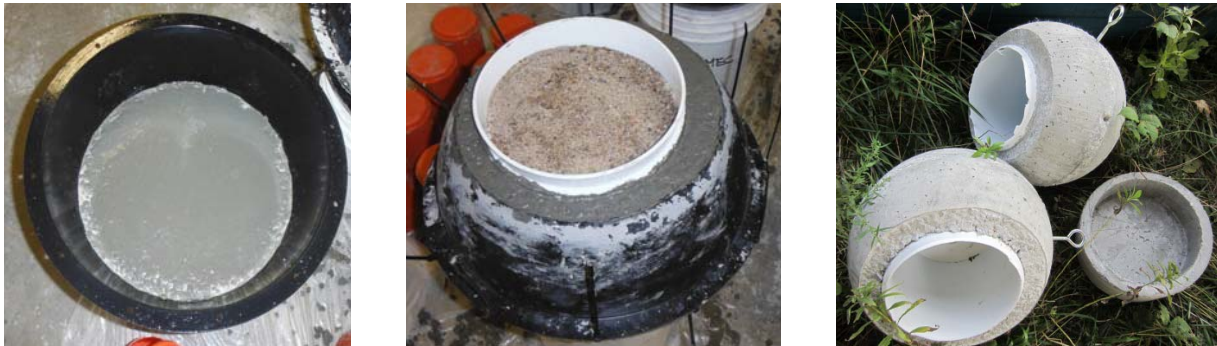
(a) Bottom half of the mold (b) Top half of the mold and cavity (c) Concrete shell and cap Fig. 9 Casting of concrete shells and caps
