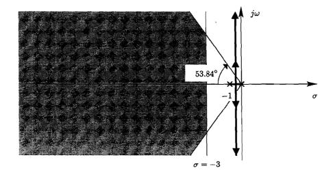
With the PI controller, we have an extra zero to pull the root-locus branches towards the desired region, where  $D(s)G(s) = K_P \frac{2(s + K_I/K_P)}{s(s+1)}.$
