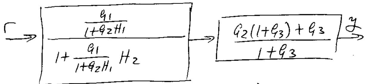
$$\frac{Y(s)}{R(s)} = \frac{q_1}{1+q_2H_1 + q_1H_2} \cdot \frac{q_2(1+q_3) + q_3}{1+q_3}$$
