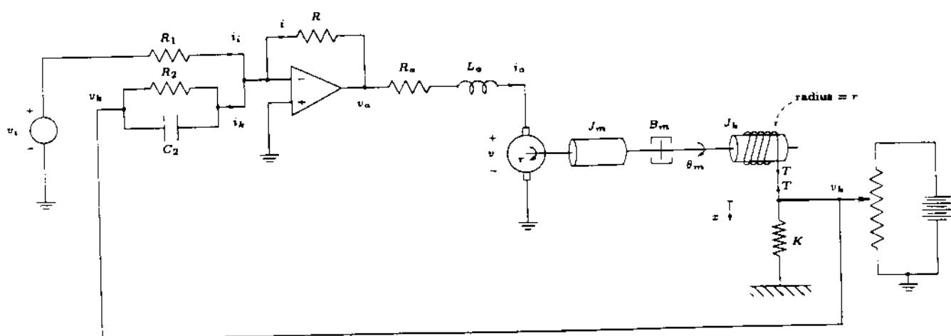
The tension on the cord is detected by the displacement  $x$ , and a variable resistor is used to obtain a voltage  $v_k$  proportional to the displacement, such that  $v_k = -k_k x$ . Draw the most detailed block diagram of the system, where  $v_i$  is the input, and  $T$  is the output. Show all the variables  $v_i, i_i, v_k, i_k, i, v_a, i_a, T, v, \theta_m, T$ , and  $x$  on the block diagram. (30pts)
