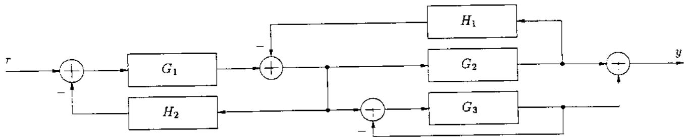
determine the transfer function *either* by block diagram reduction, *or* by Mason's formula. Show your work clearly. (25pts)
