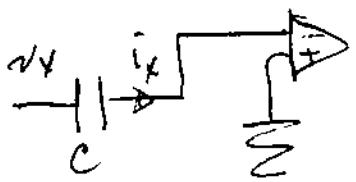
$$i_x = \frac{V_x}{R_f} = SC \frac{V_x}{\gamma_{SC}} \quad \frac{V_x}{\gamma_{SC}} \rightarrow SC i_x$$
