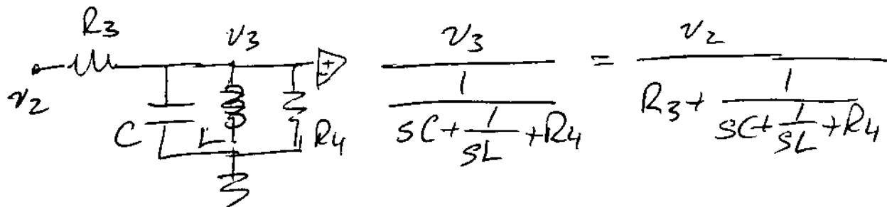
$$\frac{v_3}{\frac{1}{SC + \frac{1}{SL} + R_4}} = \frac{v_2}{R_3 + \frac{1}{SC + \frac{1}{SL} + R_4}}$$
