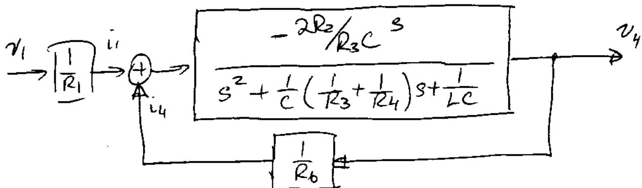
$$\frac{-2R_2/R_3C s}{s^2 + \frac{1}{C}(\frac{1}{R_3} + \frac{1}{R_4})s + \frac{1}{LC}}$$
