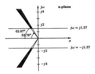
(b) Determine the largest possible 2% settling-time of a system with the poles satisfying the requirements.
