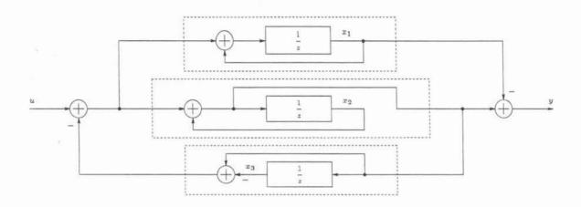
After assigning the state variables as shown in the figure, we obtain
