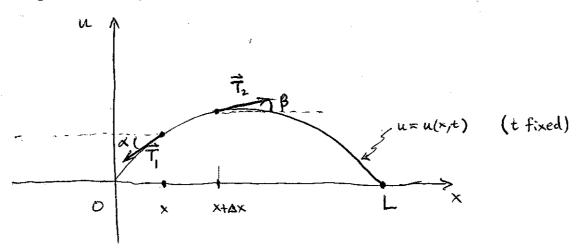
Let  $\alpha$  and  $\beta$ , respectively, denote the angles that  $T_1$  and  $T_2$  make with respect to horizontal. Then
