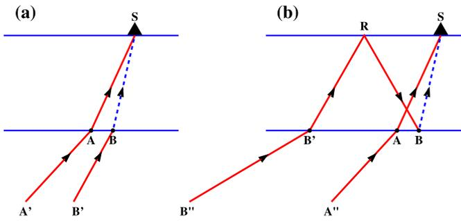
**Fig. 1.** Schematic diagrams showing the ray path of the direct P-wave (solid line segments) which pierces the discontinuity at point A, and that of the Pds (left plot) and Ppds (right plot). P-to-S conversion takes place at point B. Dashed line segments represent converted S-waves.
