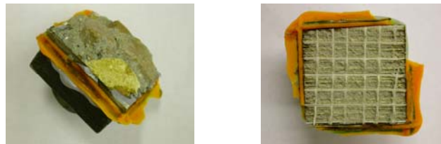
(a) SRP specimen (b) SRG specimen Figure.6. Pull-off tested specimens - failure mode
