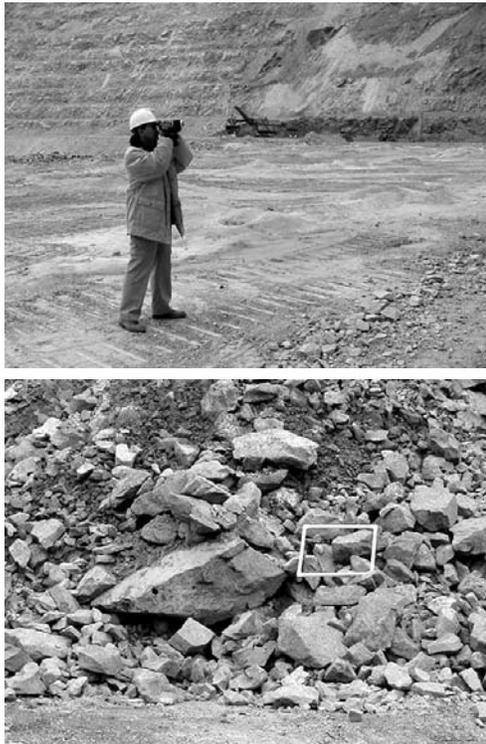
Figure 1. Image of a muck pile (bottom) taken with a roving camcorder (top); there is a scaling device in the foreground of the image.
