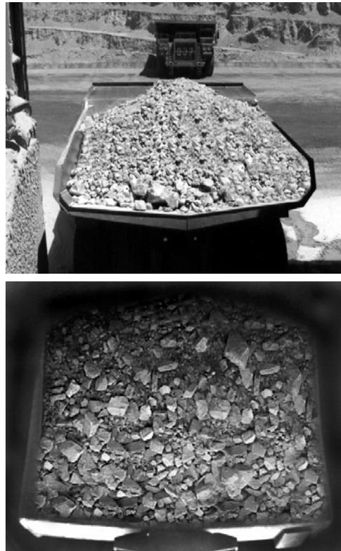
Figure 4. Image of fragmentation in back of truck (top) and in bucket of load haul (LH) vehicle (bottom).
