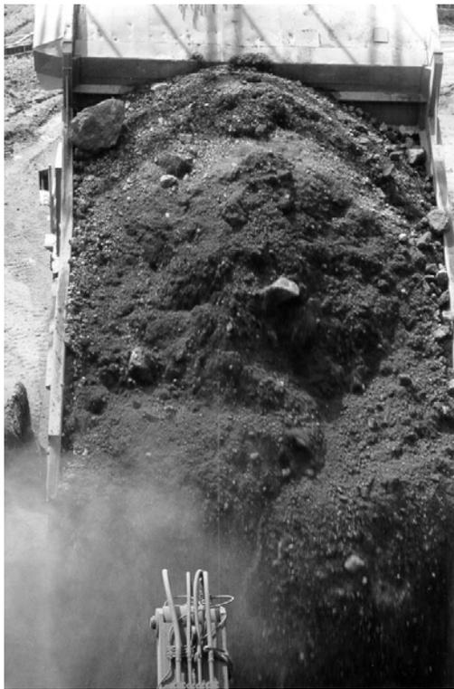
Figure 8. Truck Tipping at Hamersley Iron Ore, Australia; Early stage of dumping.
