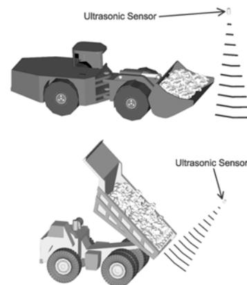
Figure 5. Use of ultrasonic sensors to determine the presence of material, either being transported (top) or dumped (bottom).
