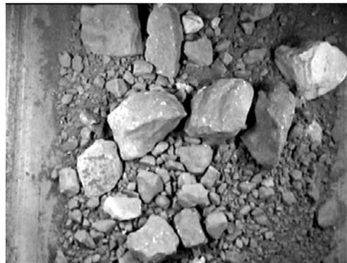
Figure 2. Imaging set-up of camera and lights (top and middle). Image of fragmentation on a conveyor belt taken with a fixed camera and fixed lighting mounted over a conveyer belt (bottom).
