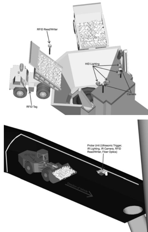
Figure 7. Camera, lighting, and RFID tag reader set-up in a position to force trucks into the correct position to be imaged.
