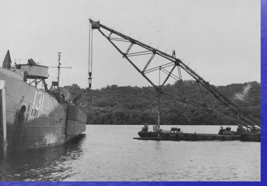
A 60-ton crane on a pontoon barge, is hoisting a pontoon causeway to lash it to the side of an LST.
