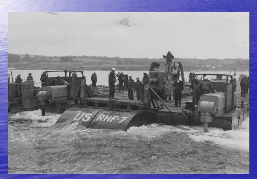
Rhino Ferries were powered by Grey-Marine 350 HP outboard motors, the largest ever made  36 Rhino Ferries were assembled from steel pontoons. They 42 ft wide and 176 ft long and fitted with a 14 by 20 ft loading ramp
