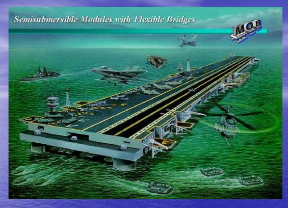
DARPA's Modular Sea Base is an emerging concept to craft a floating base from standard 20 foot ISO container size modules. The modules could be deployed from commercial containerships, would have self-contained propulsion, a means of structural interconnection, and low-level autonomy algorithms to allow sufficient flexibility in the water.
