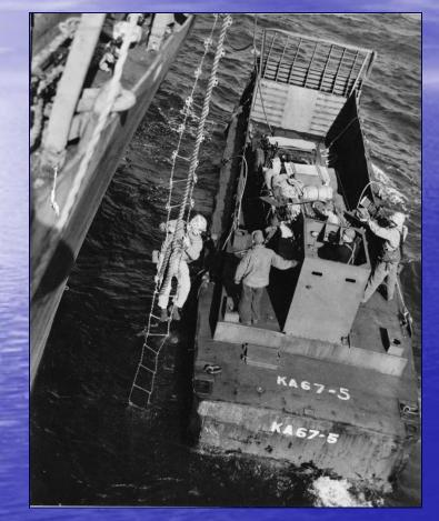
LCM's could carry Jeeps, 2-1/2 ton trucks, or even an M4 Sherman tank. They were widely employed by Seabees to ferry equipment and materials to the beachhead
