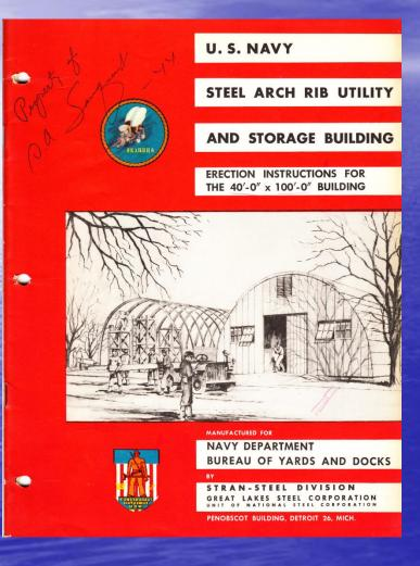
• The "Quonset 40-by-100" Arched Rib Warehouse version was developed for use at 'advance bases' (supply) Referred to as 'Elephant Huts' Used 20 tons of steel and  $\mathbf{O}$ required 650 cubic feet of shipping space in cargo holds 11,800 produced during World War II
