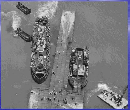
Above: An LSM is coaxed into position on a tapered pontoon 'boot blister,' while an LCT is being unloaded on the opposing blister.
