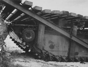
The ramps were fashioned from two 10-inch steel I-beams 25 ft long, welded to form a rectangular frame to support a flexible timber ramp
