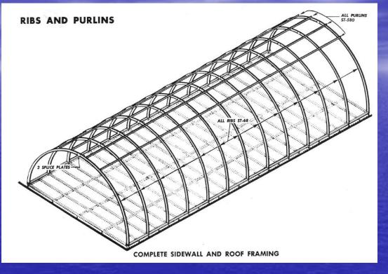
• The original Quonset Huts utilized arched ribs using steel T-sections,  $2 \times 2 \times \frac{1}{4}$  inches, and the hut was only 16 by 36 ft. These were replaced by Stran-Steel's novel ribs, which were  $2 \times 3-5/8$  inches, formed by sandwiching two lightweight channels welded back-to-back (see detail in following slide)
