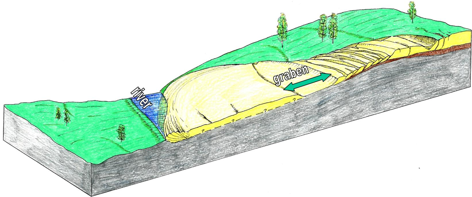
Lateral spreads are caused by liquefaction of discrete buried horizons, which allow overlying materials to “raft” towards an adjacent topographic depression, usually a body of water, such as a river, inlet or bay
