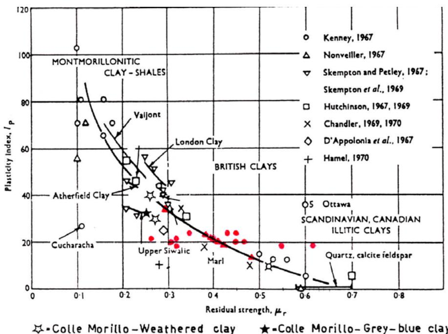
**Fig.12** - Range of residual shear strengths from actual tests on materials sampled in the Pliocene-age Orinda formation in the Mission Peak Landslide. These data plotted closer to the line of mean data because these data were derived from montmorillonitic clay shales, similar to the Orinda formation. .
