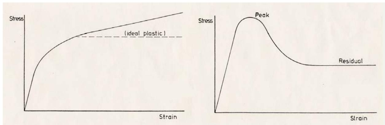
**Fig. 1** presents the stress-strain behavior of two varying geologic materials involved in landslippage. The left diagram presents stress-strain behavior of a quasi-plastic, or *strain-hardening material*, such as normally consolidated clay. The right-hand plot shows the behavior exhibited by brittle materials, such as overconsolidated clay or bedrock, which tend to exhibit *strain-softening behavior*.
