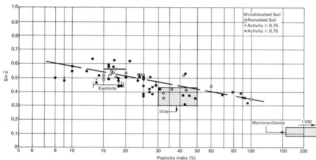
**Figure 8 – Relationship between  $\sin \phi'$  and plasticity index for normally consolidated soils, using data from Kenney (1959) and Olson (1974). Note how montmorillonitic clay plots off the chart to right.**
