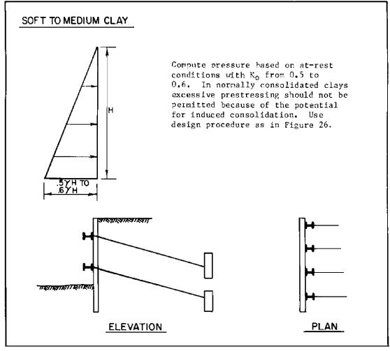
FIGURE 29 Pressure Distribution for Tied-Back Walls
