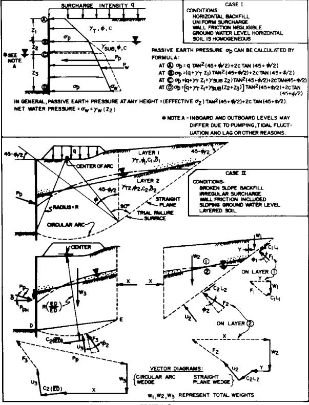
FIGURE 9 Computation of General Passive Pressures
