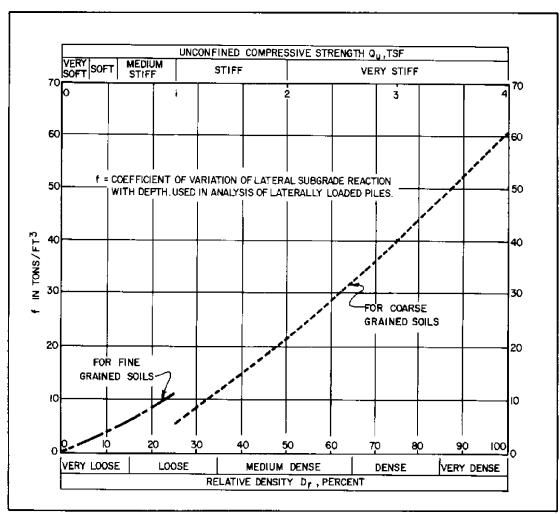
FIGURE 9 Coefficient of Variation of Subgrade Reaction
