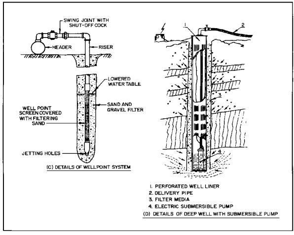
FIGURE 13 (continued) Methods of Construction Dewatering
