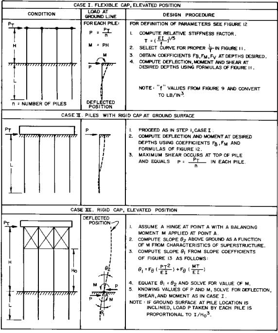
FIGURE 10 Design Procedure for Laterally Loaded Piles
