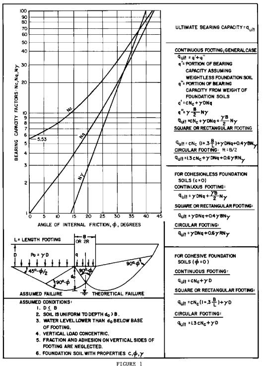
Ultimate Bearing Capacity of Shallow Footings With Concentric Loads 7.2-131
