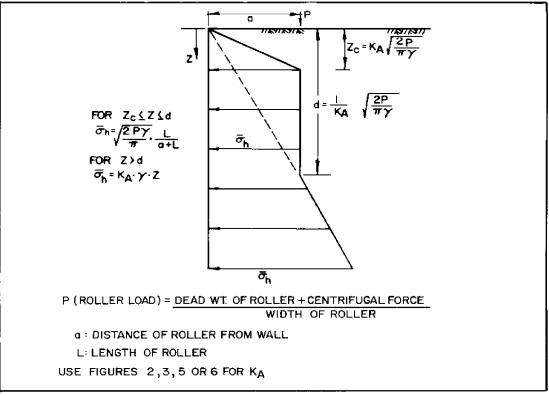
FIGURE 13 Horizontal Pressure on Walls from Compaction Effort
