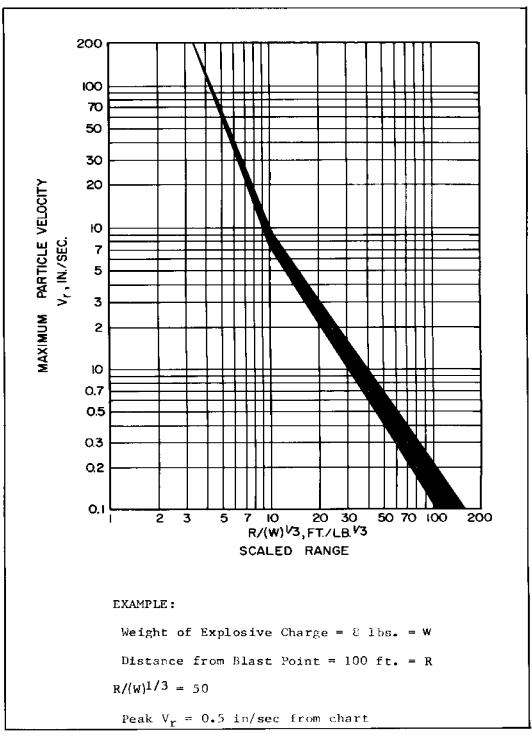
FIGURE 10 Cube Root Scaling Versus Maximum Particle Velocity
