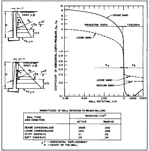
FIGURE 1 Effect of Wall Movement on Wall Pressures
