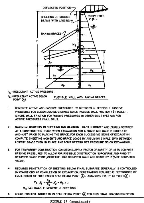
FIGURE 27 (continued) Design Criteria for Braced Flexible Walls
