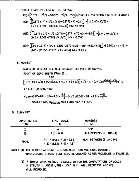
FIGURE 31 (continued) Example of Excavation in Stages
