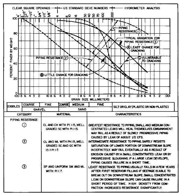
FIGURE 1 Resistance of Earth Dam Embankment Materials To Piping and Cracking
