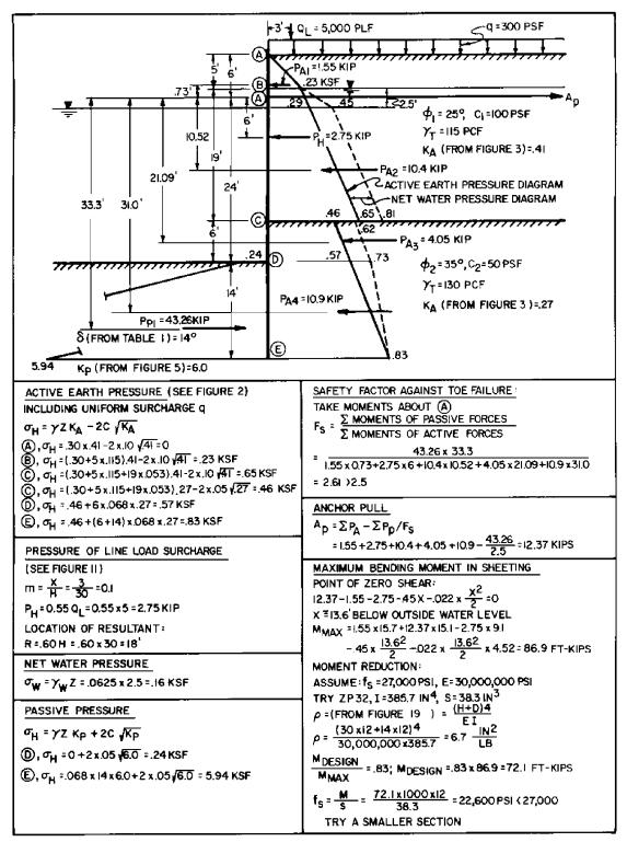
FIGURE 21 Example of Analysis of Anchored Bulkhead
