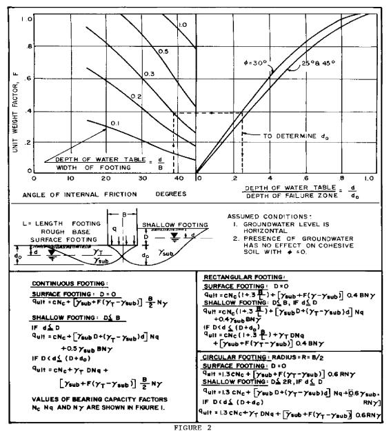
Ultimate Bearing Capacity With Groundwater Effect
