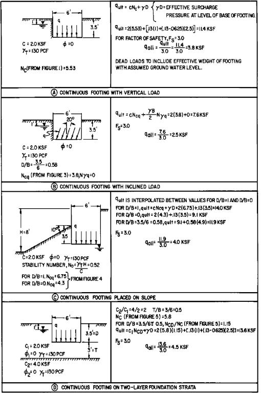
FICURE 6 Examples of Computation of Allowable Searing Capacity Shallow Footings on Cobesive Scils
