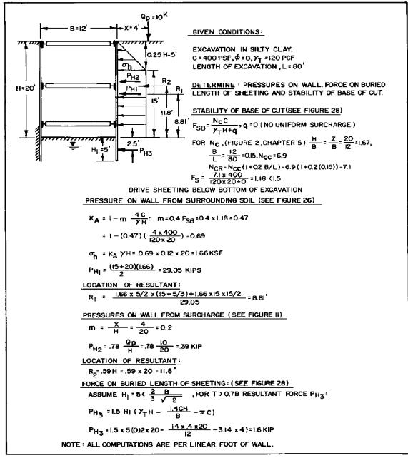
FIGURE 30 Example of Analysis of Pressures on Flexible Wall of Narrow Cut In Clay - Undrained Conditions
