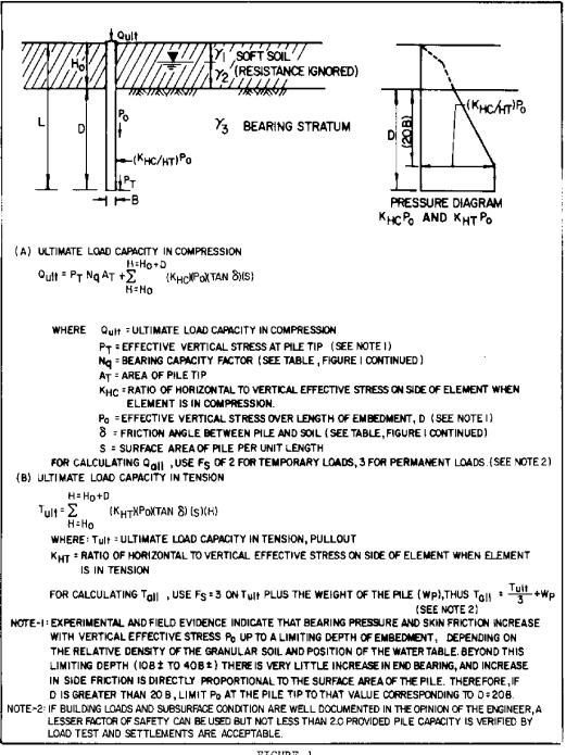
FIGURE 1 Load Carrying Capacity of Single Pile in Granular Soils
