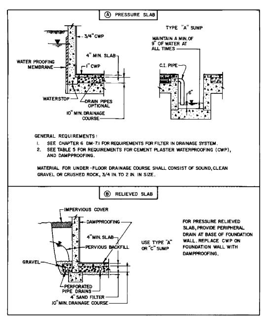
FIGURE 15 Typical Foundation Drainage and Waterproofing
