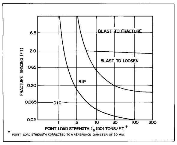
FIGURE 9 Suggested Guide for Ease of Excavation
