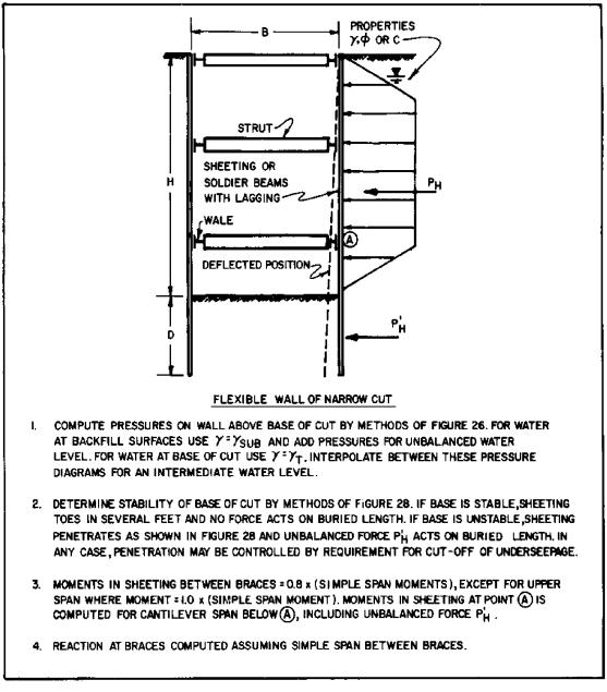
FIGURE 27 Design Criteria for Braced Flexible Walls
