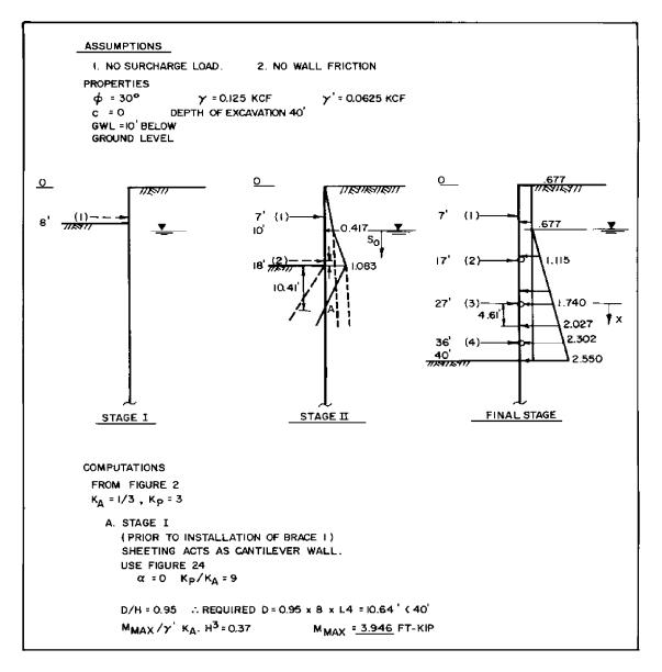
FIGURE 31 Example of Excavation in Stages
