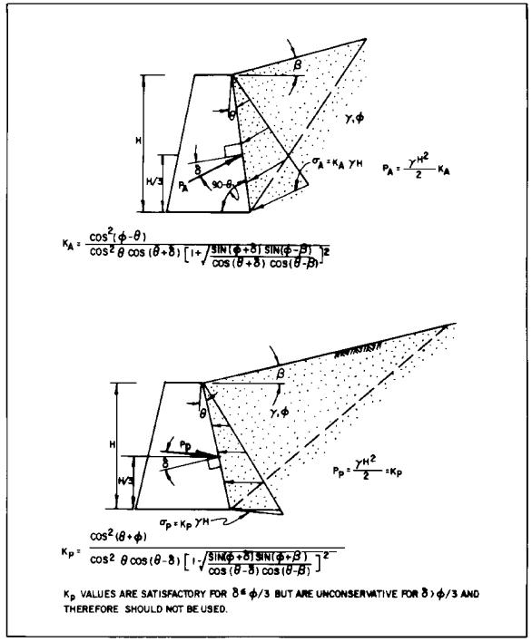
FIGURE 8 Coefficients  $K_{\rm A}$  and  $K_{\rm p}$  for Walls with Sloping Wall and Friction, and Sloping Backfill
