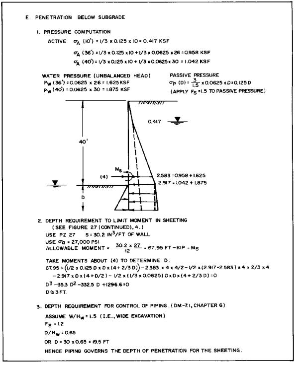
FIGURE 31 (continued) Example of Excavation in Stages
