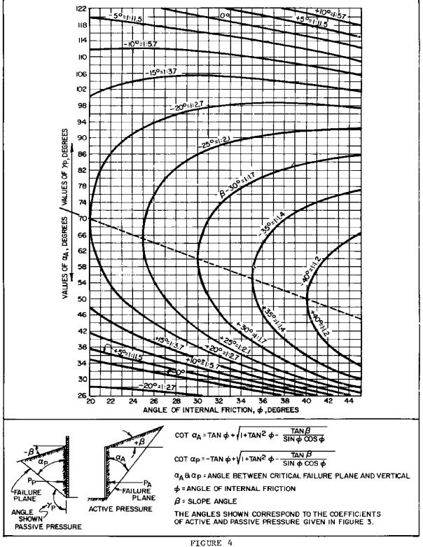
FIGURE 4 Position of Failure Surface for Active and Passive Wedges (Granular Soils) 7.2-65
