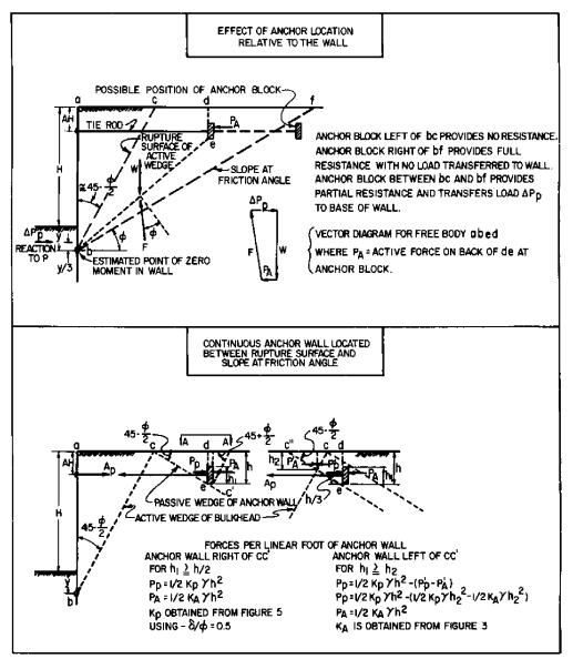
FIGURE 20 Design Criteria for Deadman Anchorage
