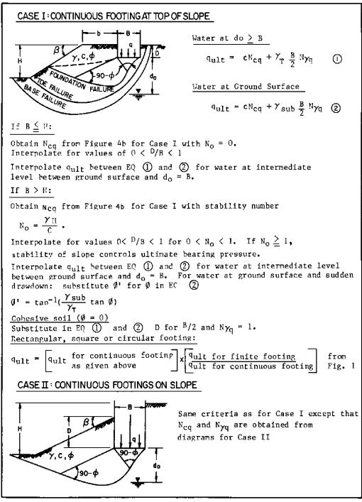
FIGURE 4a Ultimate Bearing Capacity For Shallow Footing Placed on or Near a Slope
