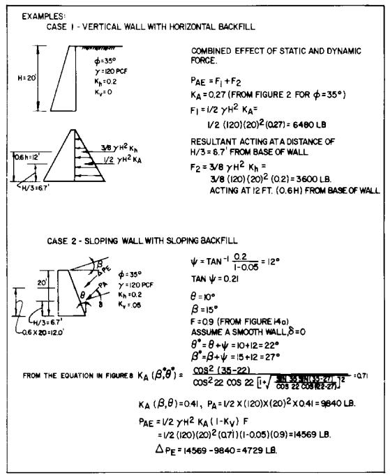
FIGURE 14(b) Example Calculations for Dynamic Loading on Walls
