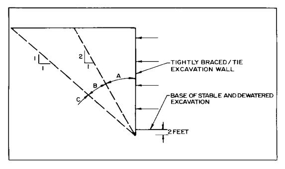
FIGURE 7 General Guidance for Underpinning
