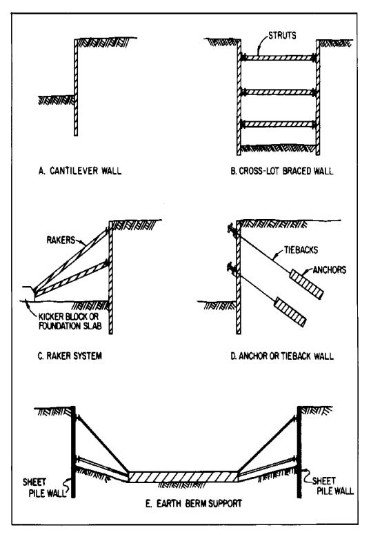
FIGURE 6 Support System - Walled Excavation
