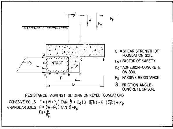
FIGURE 15 (continued) Design Criteria for Rigid Retaining Walls
