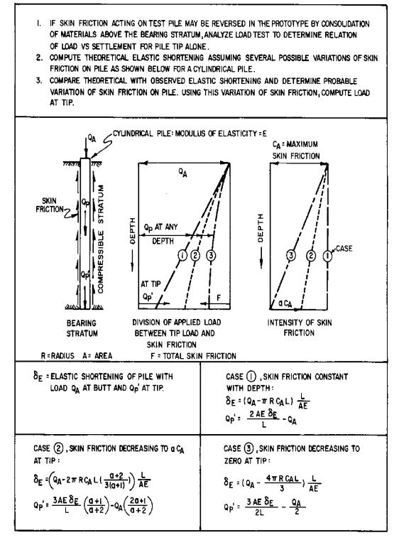
FIGURE 7 Load Test Analysis Where Downdrag Acts on Pile
