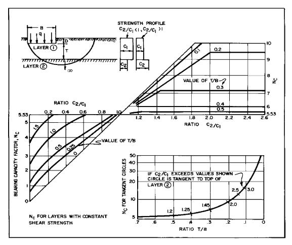
FIGURE 5 Ultimate Bearing Capacity of Two Layer Cohesive Soil ( $\emptyset$ =0)
