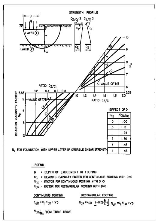
FIGURE 5 (continued) Ultimate Bearing Capacity of Two Layer Cohesive Soil (Ø=0)
