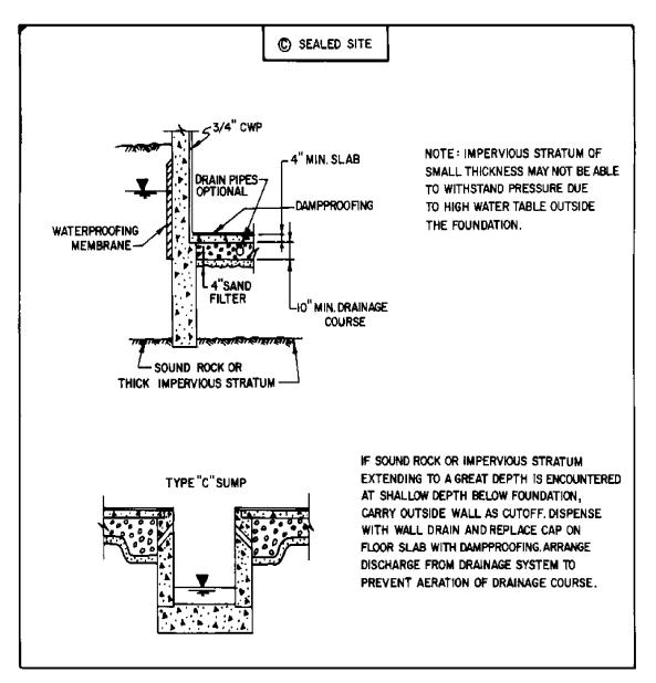
FIGURE 15 (continued) Typical Foundation Drainage and Waterproofing
