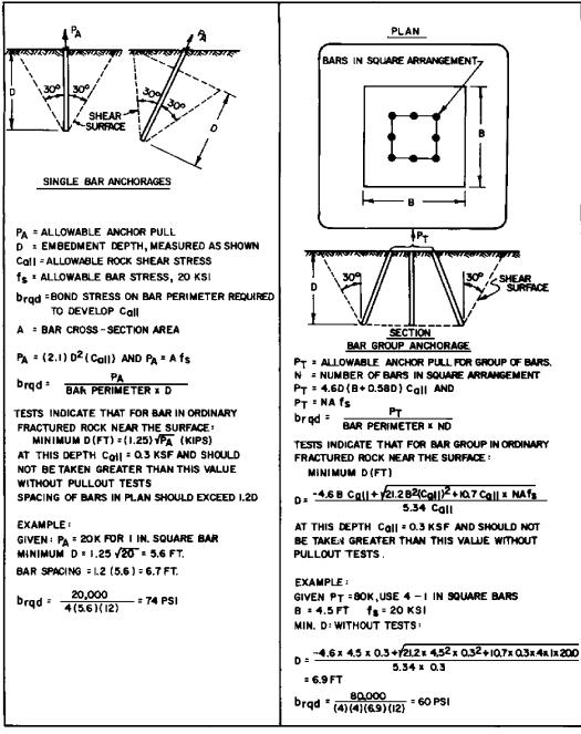
FIGURE 16 Capacity of Anchor Rods in Fractured Rock
