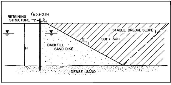
FIGURE 22 Sand Dike Scheme for Controlling Active Pressure
