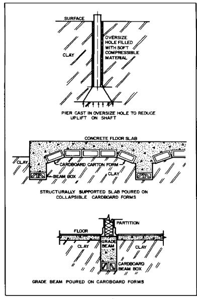
FIGURE 14 Construction Details for Swelling Soils
