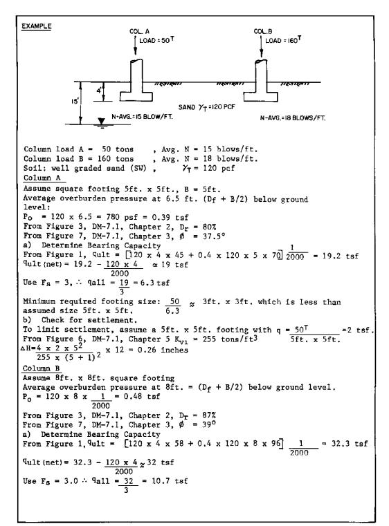
FIGURE 9 Example of Proportioning Footing Size to Equalize Settlements 7.2-148
