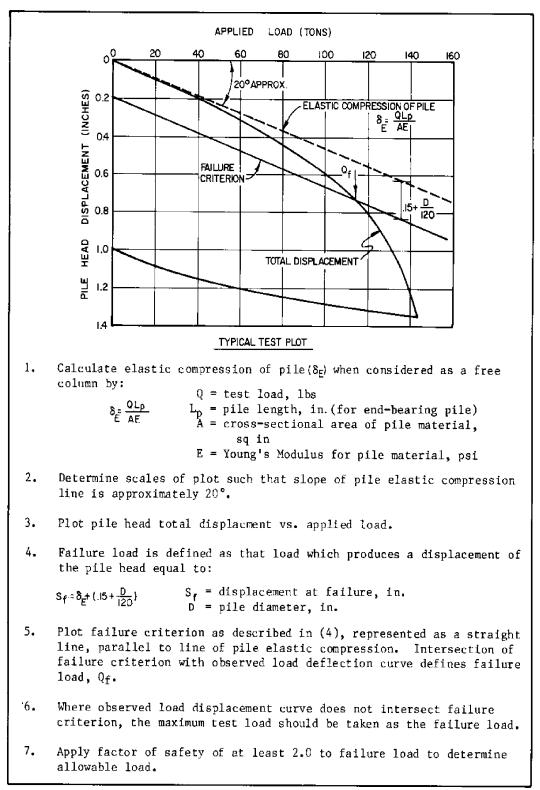
FIGURE 6 Interpretation of Pile Load Test
