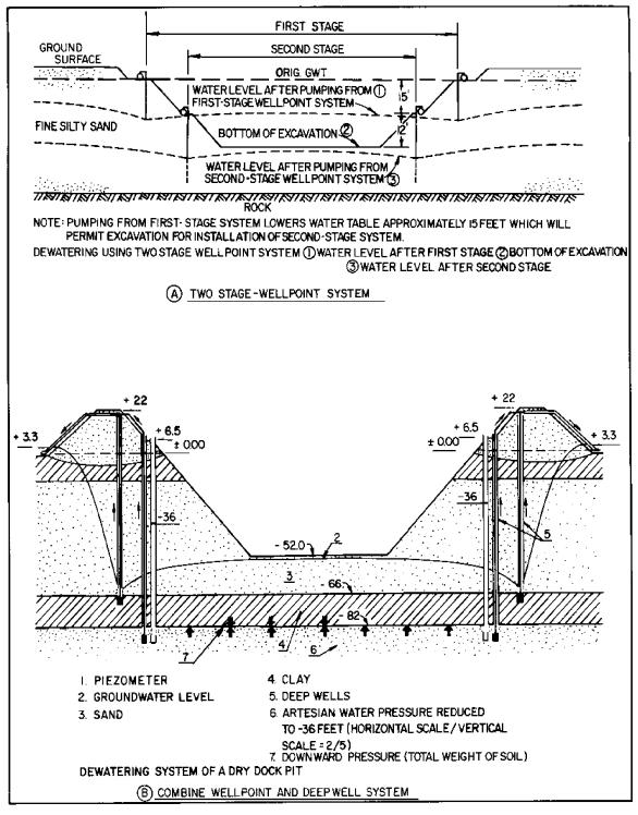
FIGURE 13 Methods of Construction Dewatering
