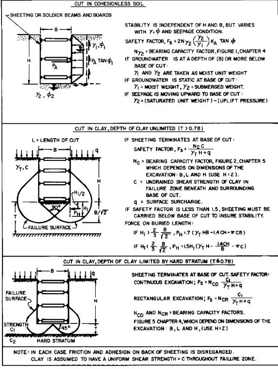
FIGURE 28 Stability of Base for Braced Cut
