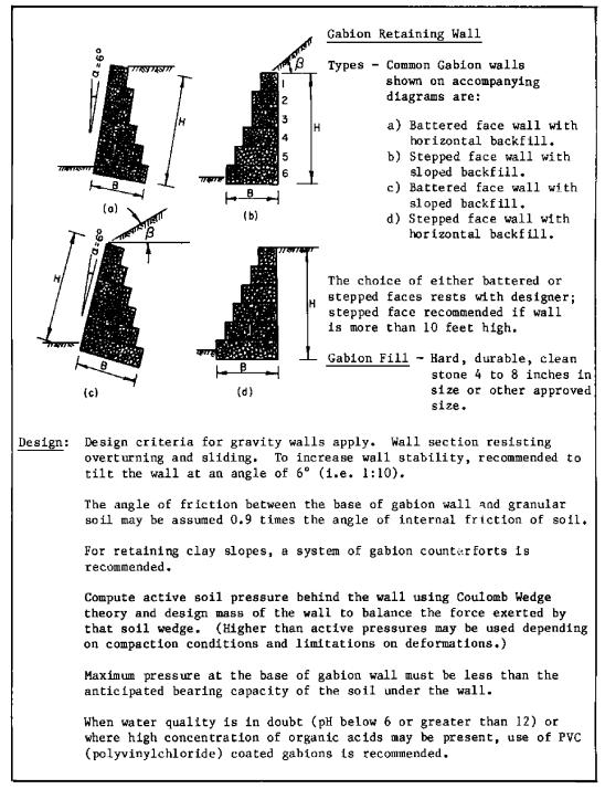
FIGURE 34 Gabion Wall
