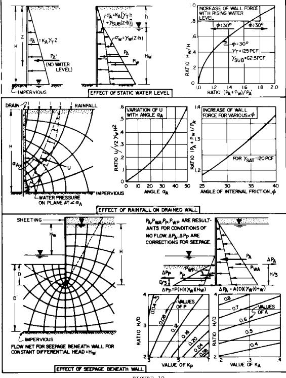
FIGURE 10 Effect of Groundwater Conditions on Wall Pressures
