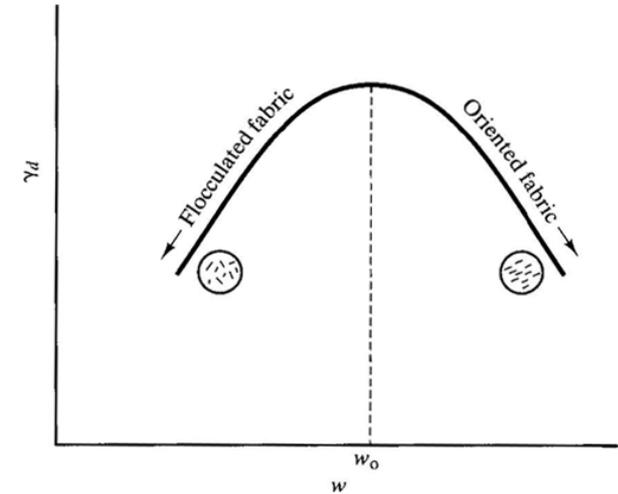
Soils “dry” of optimum moisture tend to be more flocculated, with a “cardhouse” fabric. Soils compacted “wet” of optimum moisture tend to be more compact, with lower void ratio
