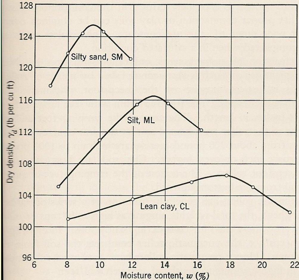
Fig. 171. Standard Proctor compaction curves.
