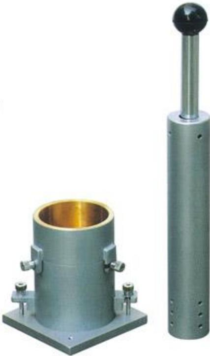
Standard Proctor Compaction Mold with collar extension and drop hammer in cylindrical sleeve
