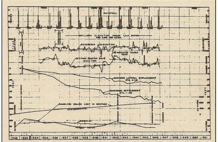
Form used to show 20 years record of rainfall, reservoir stages, seepage, lateral displacement and settlement of crest of dam, and dissolved solids in seepage water, together with earthquake, repair, grouting and related data.
