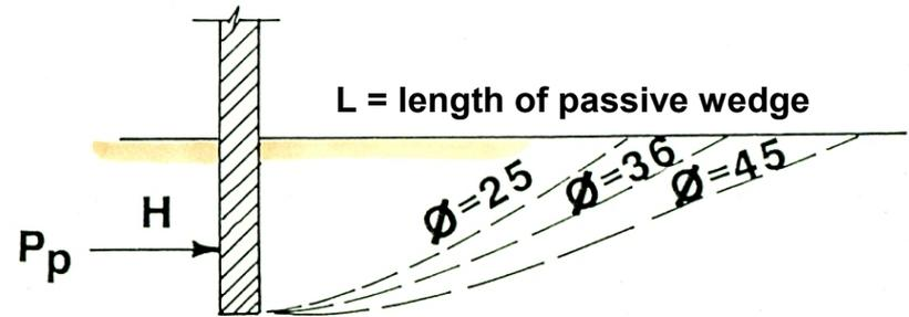
**Ratio of length-to-height for passive soil resistance wedges on resisting side of cantilever elements, as a function of soil friction,  $\phi$ . Note that the normal range is something between 2 and 4.**
