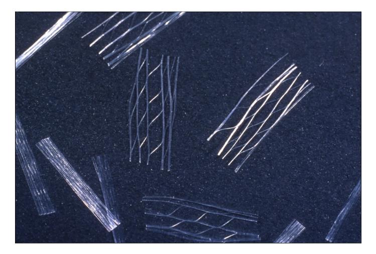
Geofibers© are expandable polyproylene strands that are mixed with soils to increase their shear strength. Typical mixtures vary between 0.1 and 0.4% by weight.
