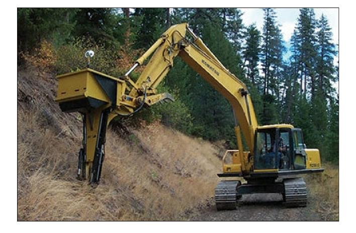
An expandable stinger attached to an excavator boom, as shown above, can plant nursery stock on steep slopes or in riprap (image from Dan Culley of Dayton Tractor & Crane Co., via FHWA)
