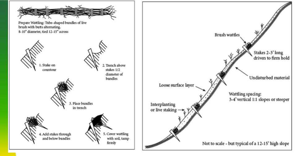
Live Willow wattles are prepared by wrapping tubeshaped bundles with alternating butts (left), then staking these into shallow trenches and covering with loose soil, as shown at left and right.
