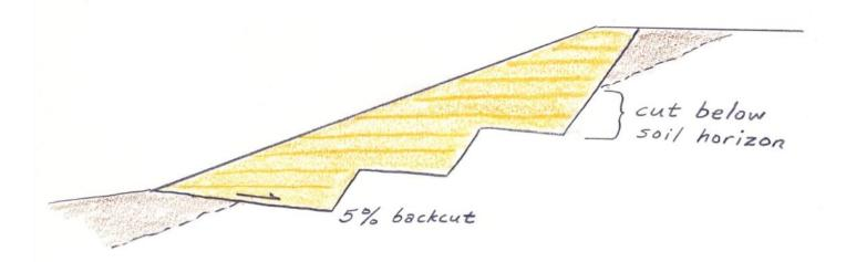
Shear keys are intended to remove compressible fine grained, low permeability soils and provide additional mechanical interlocking with the subgrade. They were initially codified in the Los Angeles Grading Ordinance of 1952
