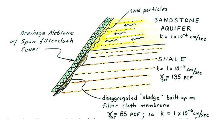
Drainage membranes with filter fabrics may appear to become clogged with silt, or "sludge" on their upgradient side. But this sludge is always more permeable (lower density) than the parent material from which it emanates.
