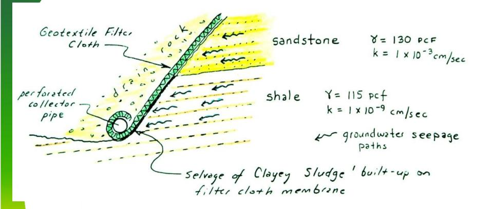
Filter cloths prevent infiltration of fines into subdrain media. A selvage of fine grained sludge can be expected to accumulate against the filter cloth, but this should not prevent infiltration
