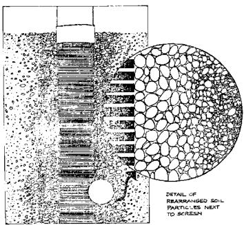
Slotted casings are normally employed as well screens within the aquifers being taped by water wells. The width of the slots should allow 50 to 60% of the sand grains to enter the well and be removed, creating an inverted filter (see drawing above). An envelope of well graded granule gravel & coarse sand is usually placed around the casing.
