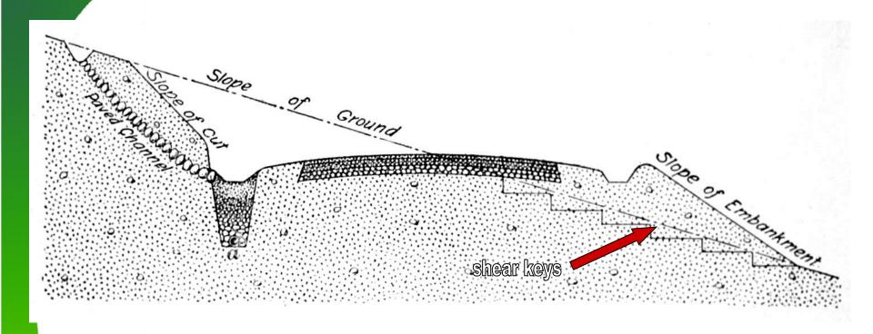
Shear keys have been recognized as an integral component of sidehill embankments for hundreds of years! This shows a typical section for a textbook published in 1893.
