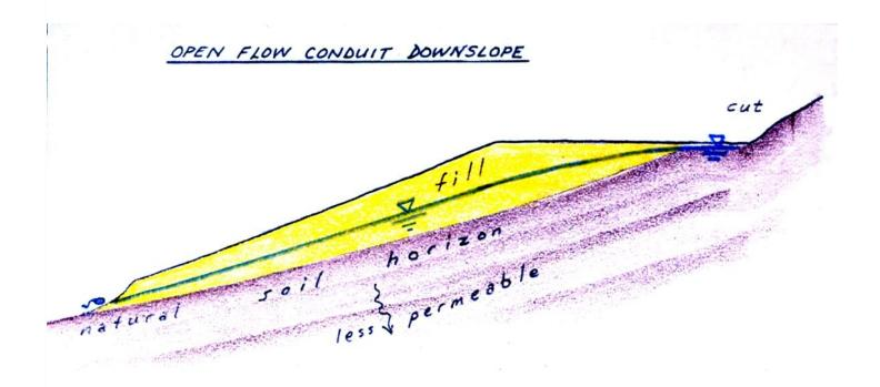
With time, the underlying soils will consolidate under the fill surcharge and the coarse layer at the base of the fill gradually becomes clogged by the root mat that tends to grow around the seepage outfall at the base of the fill.
