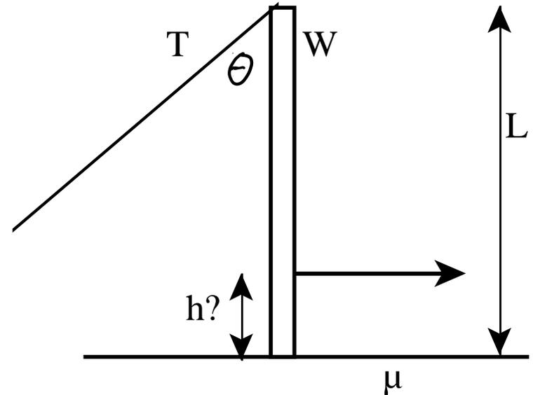
Derive an expression for the height  $h$  above the ground at which the pulling force is applied, in terms of relevant system parameters.
