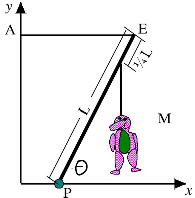
Derive an expression for the tension in the horizontal cable **AE**.
