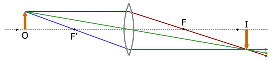
object between f and 2f: image is real, inverted, enlarged object outside of 2f: image is real, inverted, reduced object inside of f: image is virtual, upright, enlarged
