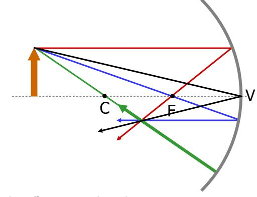
Ray 4 goes to the vertex V and reflects under the same angle below the optical axis
