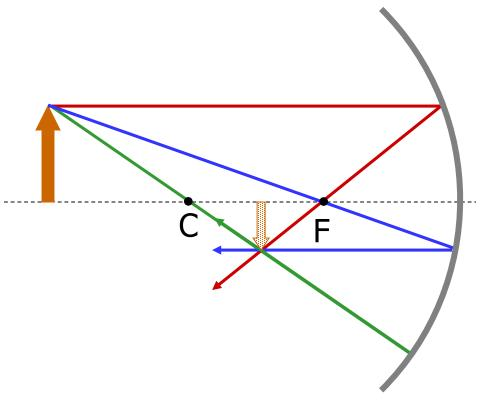
Real image: outgoing rays do cross. Can be captured on screen or by camera.
