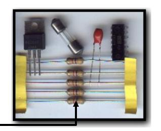
The little bands of color on the resistors have meaning. Here are a couple of handy web links:
