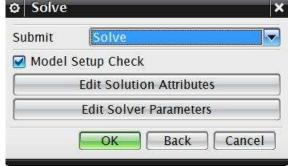
It may take a while to generate the results. Wait until the **Analysis Job Monitor** window appears, showing the job to be **Completed**. While the solver is doing computations, the **Analysis Job Monitor** will show as **Running**
