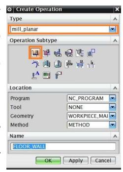
In flooring operations, it is always better to keep the Stepover value to be less than half of the diameter of the cutter in order to achieve more
